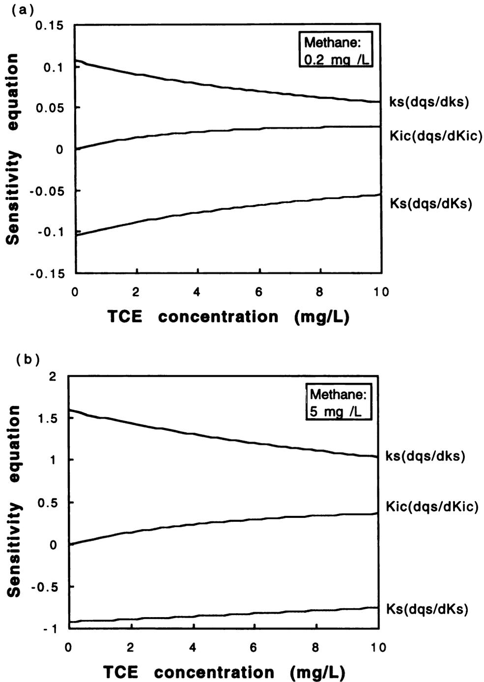
Figure. 5.6 Sensitivity equation for  $q_s$  as a function of TCE concentration for methanotrophic mixed culture at a specified methane concentration.
