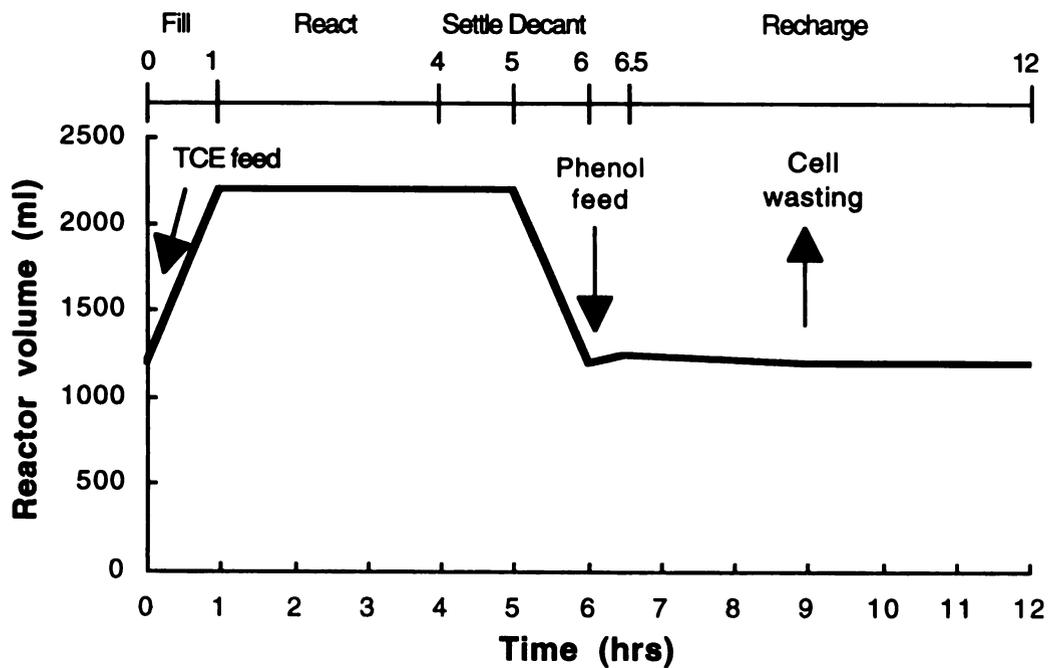
Figure 7.2. The operating mode of SBR in a cycle
