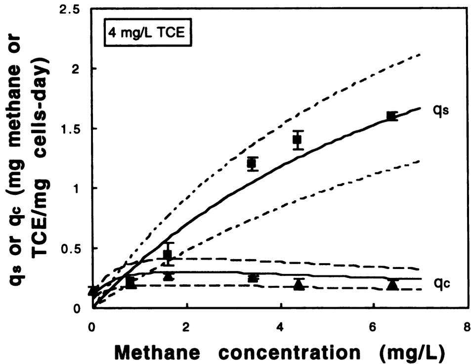
Figure 4.5 The effect of methane concentration on TCE and methane degradation rate when both substrates are present at same time. (a) Initial concentration of TCE is 8 mg/L and (b) Initial concentration of TCE is 4 mg/L. Error bars indicate 95% confidence interval. Dashed lines indicate error range for the prediction.
