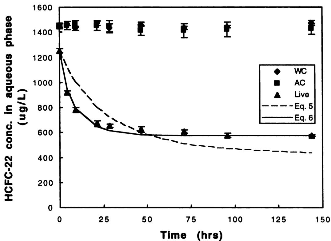
Figure 3.1 Biotransformation of HCFC-22 by methanotrophic mixed culture MM1. Fitting parameters are summarized in Tables 3.4 and 3.5. Error bars give standard deviations for three samples. WC = water control (no cells), AC = autoclaved control, LIVE = 275 mg/L MM1 (dry weight).
