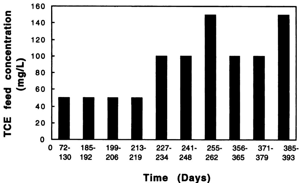
Figure 6.2. TCE feed concentration for long-term TCE exposure experiment in chemostat
