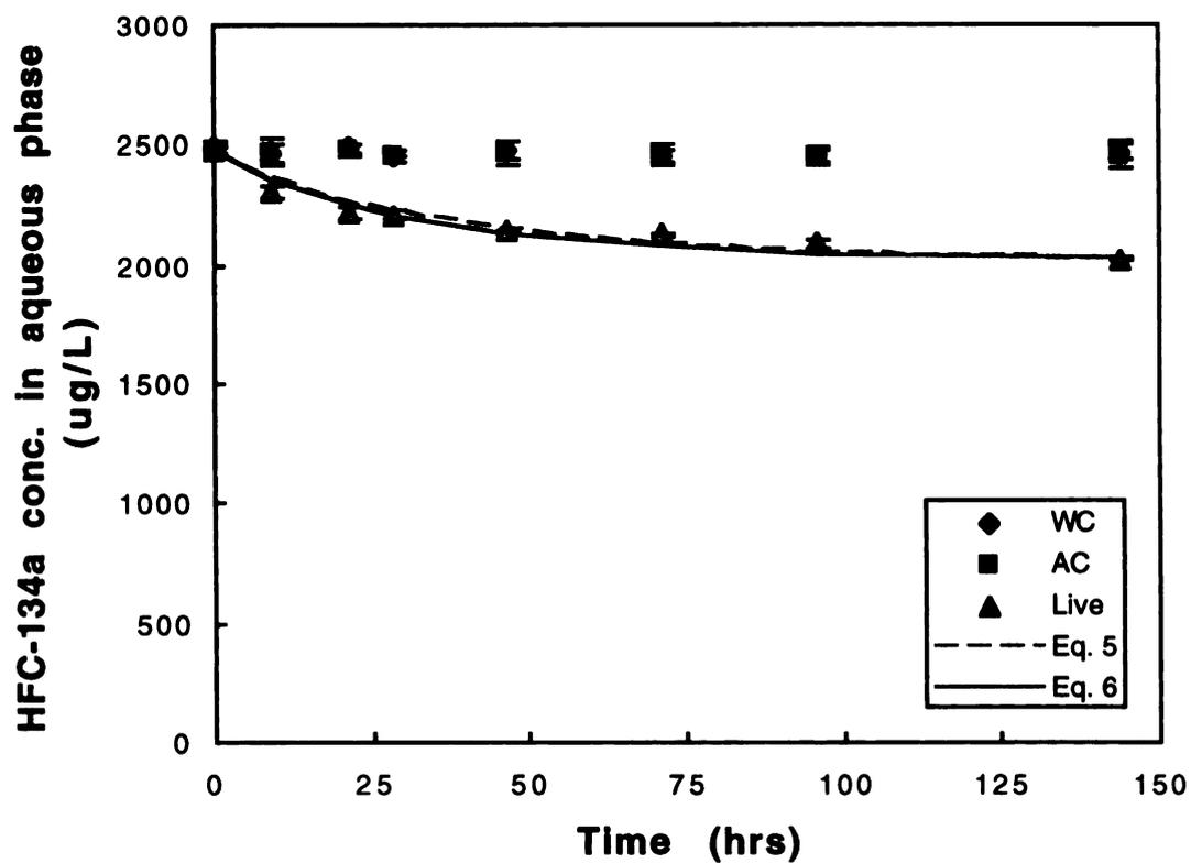
Figure 3.3 Biotransformation of HFC-134a by methanotrophic mixed culture MM1. Fitting parameters are summarized in Tables 3.4 and 3.5. Error bars give standard deviations for three samples. WC = water control (no cells), AC = autoclaved control, LIVE = 275 mg/L MM1.
