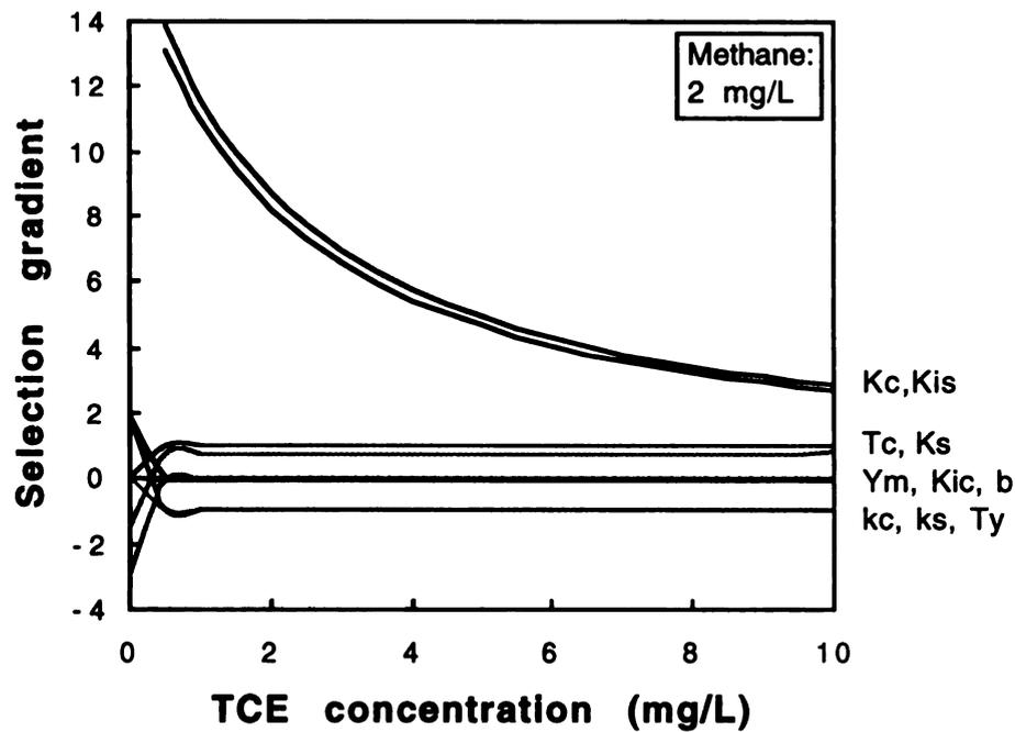
Figure. 5.4 Dimensionless selection gradient,  $(P/W)(\partial W/\partial P)$  as a function of TCE concentration for methanotrophic mixed culture at a specified methane concentration.
