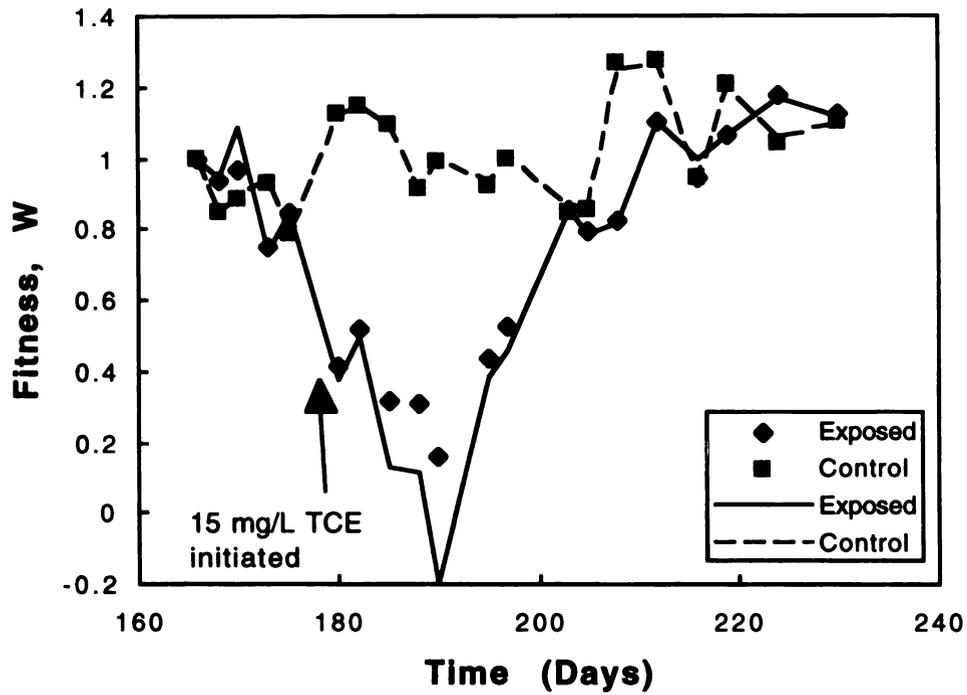
Figure 7.7 Fitness of phenol-degrading communities during period when the exposed reactor received an influent concentration 25 mg/L TCE. Fitness calculations are based on  $\mu$  measurements ( $\diamond$ ,  $\bullet$ ) and fitness components ( $—$ ,  $---$ ), respectively.
