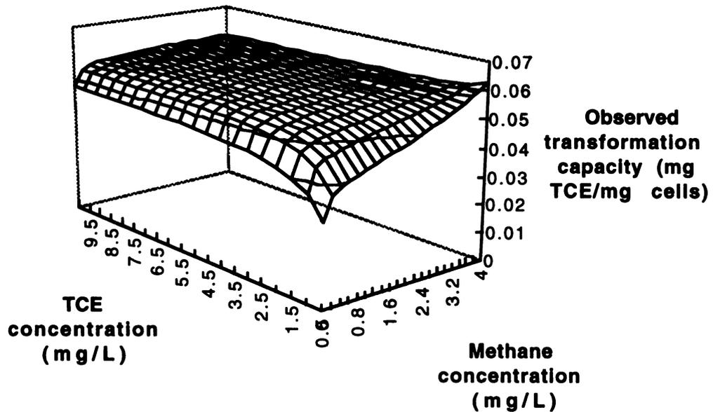
Figure 4.6 The observed transformation capacity as a function of the concentrations of growth and nongrowth substrates. Prediction is based on parameters listed in Table I.
