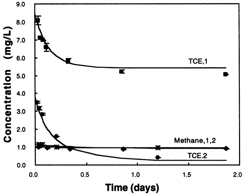
Figure 4.4 Biotransformation of TCE and methane by methanotrophic mixed culture: comparison with model prediction (for different initial TCE concentration). Error bars indicate the 95% confidence interval for triplicate samples.
