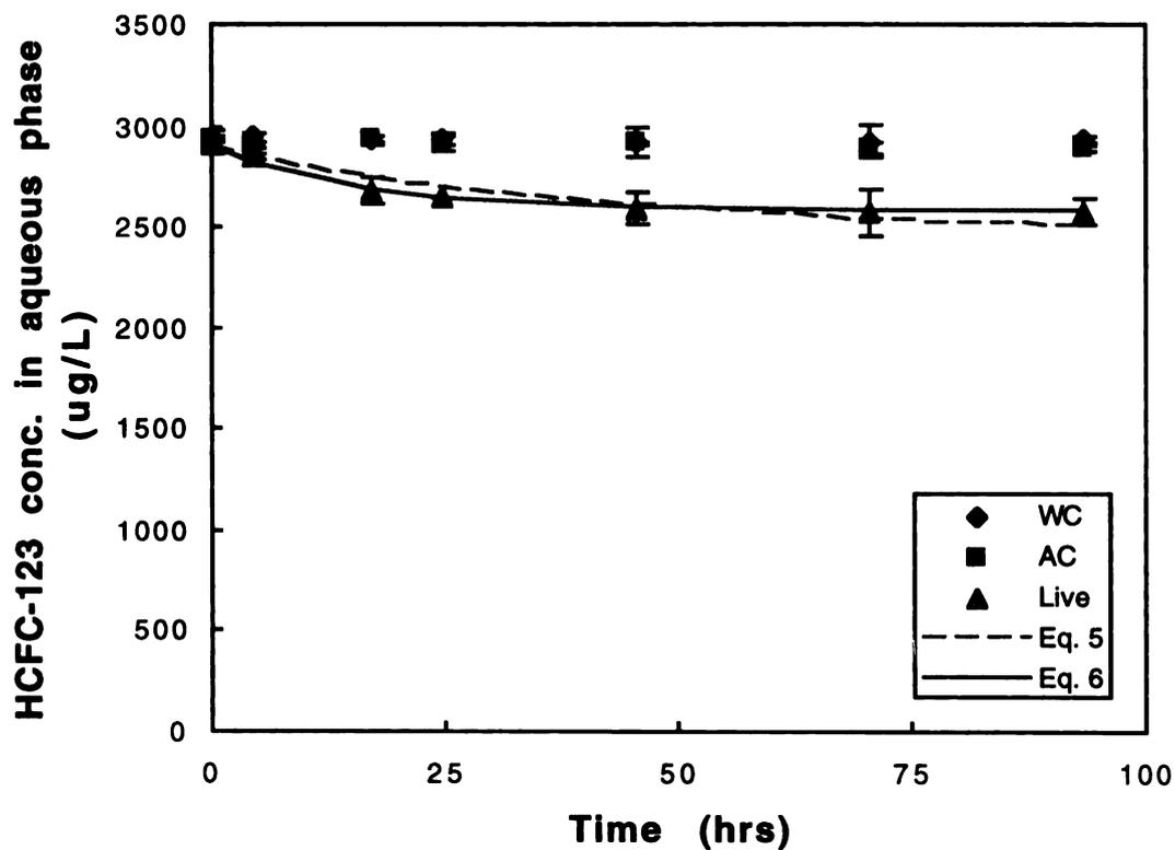
Figure 3.4. Biotransformation of HCFC-123 by methanotrophic mixed culture MM1. Fitting parameters are summarized in Tables 3.4 and 3.5. Error bars give standard deviations for three samples. WC = water control (no cells), AC = autoclaved control, LIVE = 275 mg/L MM1.
