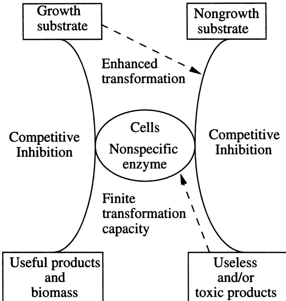
Figure 1.2 General scheme of cometabolic transformation. Dashed lines indicate the effects of substrates or products on transformation.
