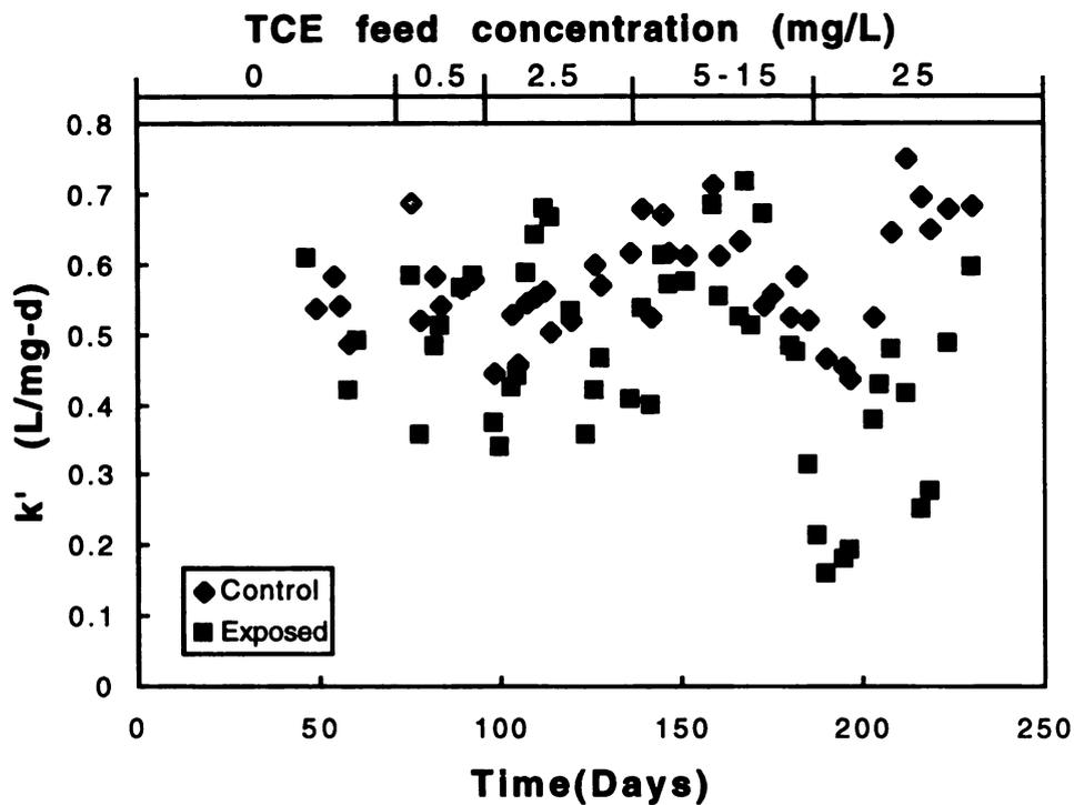
Figure 7.4 Second order rate coefficients of TCE transformation by phenol-degrading reactor communities.
