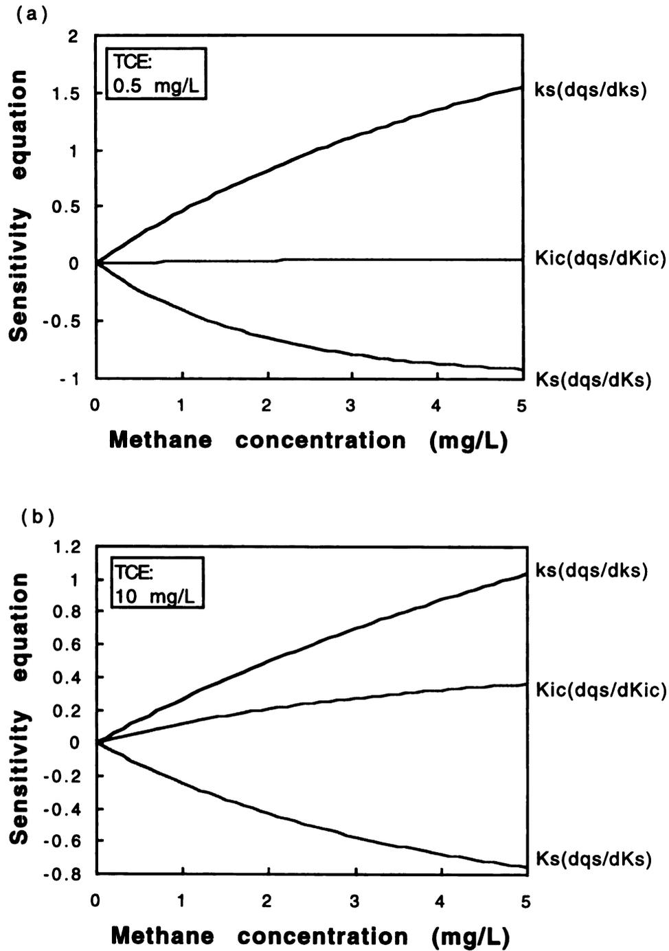
Figure. 5.7 Sensitivity equation for  $q_s$  as a function of methane concentration for methanotrophic mixed culture at a specified TCE concentration.
