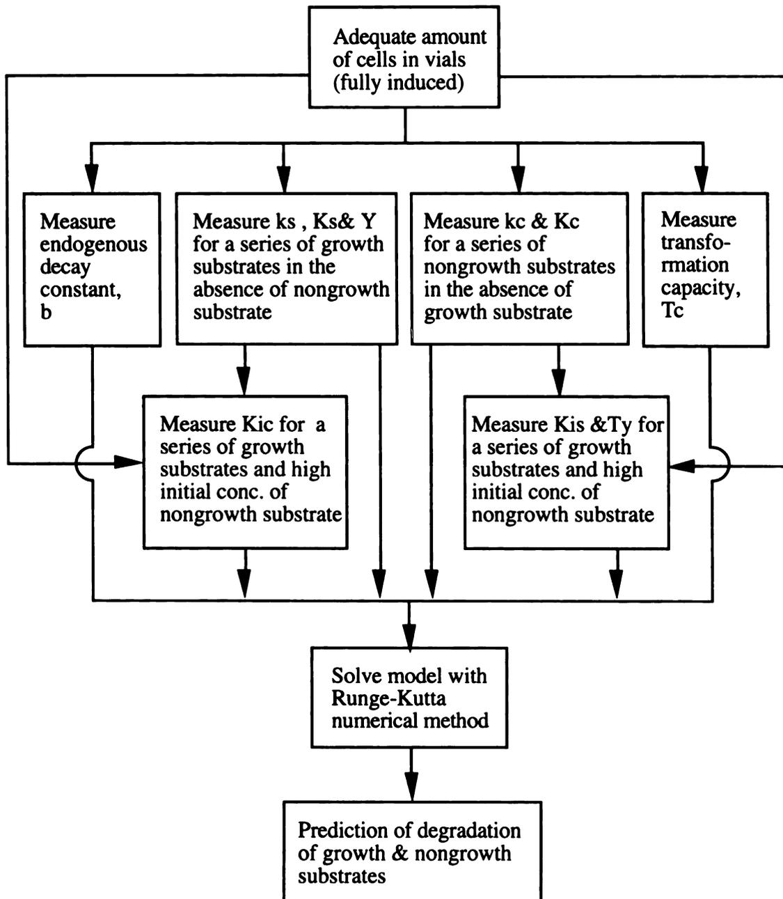
Figure 4.1 Approach for prediction of degradation of growth and nongrowth substrates by the proposed model.
