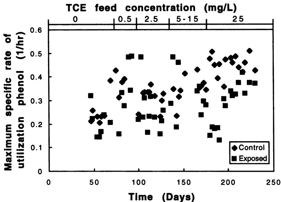
Figure 7.5 Maximum specific rate of phenol utilization by phenol-degrading reactor communities.
