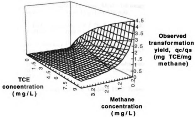
Figure 4.7 The observed transformation yield as a function of the concentration of growth and nongrowth substrates. Prediction is based on parameters listed in Table I.
