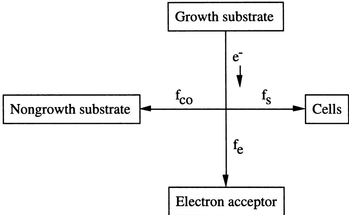
Figure 1.1 Flow of reducing power in cometabolizing system
