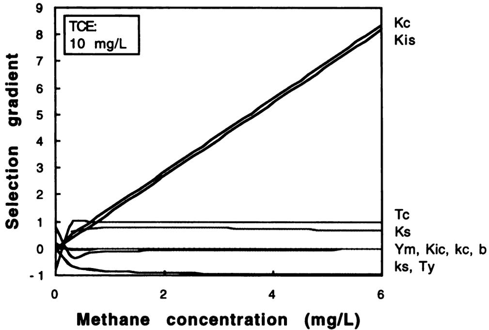
Figure. 5.5 Dimensionless selection gradient,  $(P/W)(\partial W/\partial P)$  as a function of methane concentration for methanotrophic mixed culture at a specified TCE concentration.
