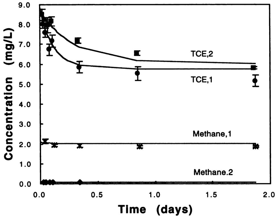
Figure 4.3 Biotransformation of TCE and methane by methanotrophic mixed culture: comparison with model predictions (for different initial methane concentration). Error bars indicate the 95% confidence interval for triplicate samples.
