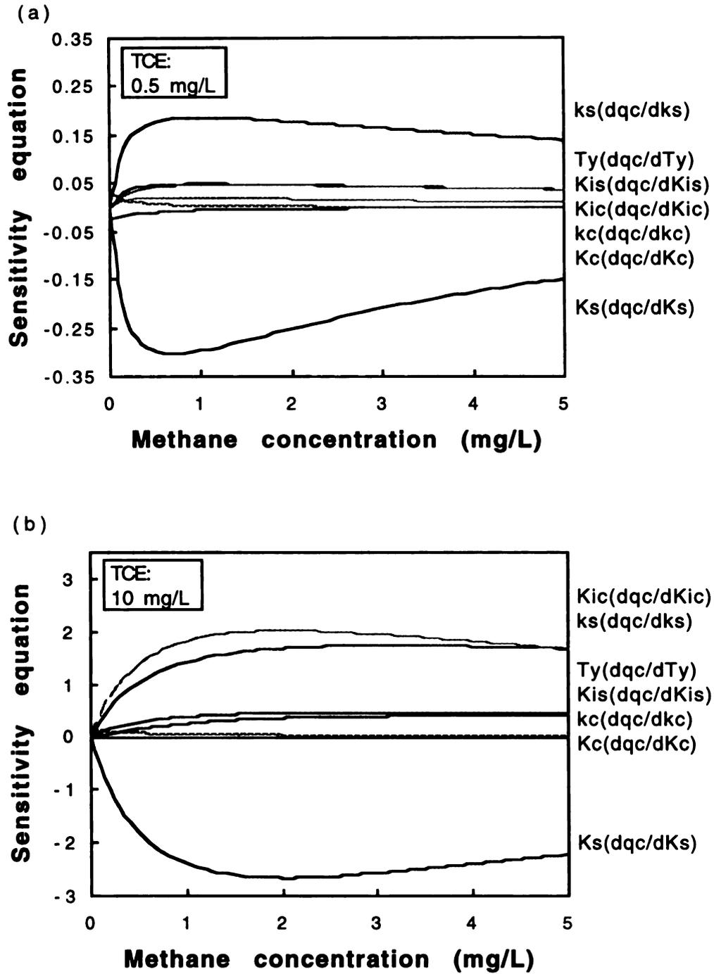
Figure. 5.9 Sensitivity equation for  $q_c$  as a function of methane concentration for methanotrophic mixed culture at a specified TCE concentration.
