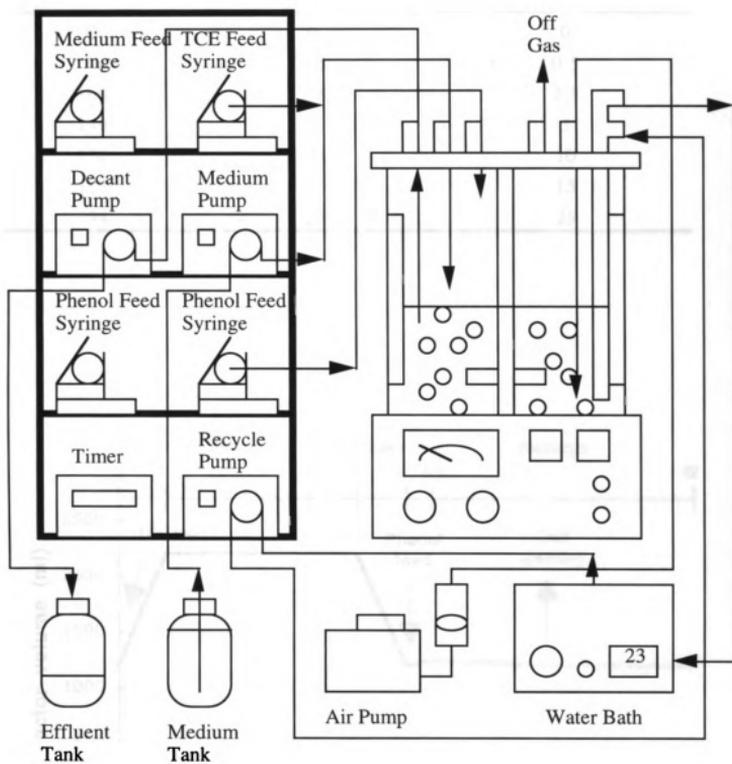
Figure 7.1. Experimental setup for bench-scale sequencing batch reactors
