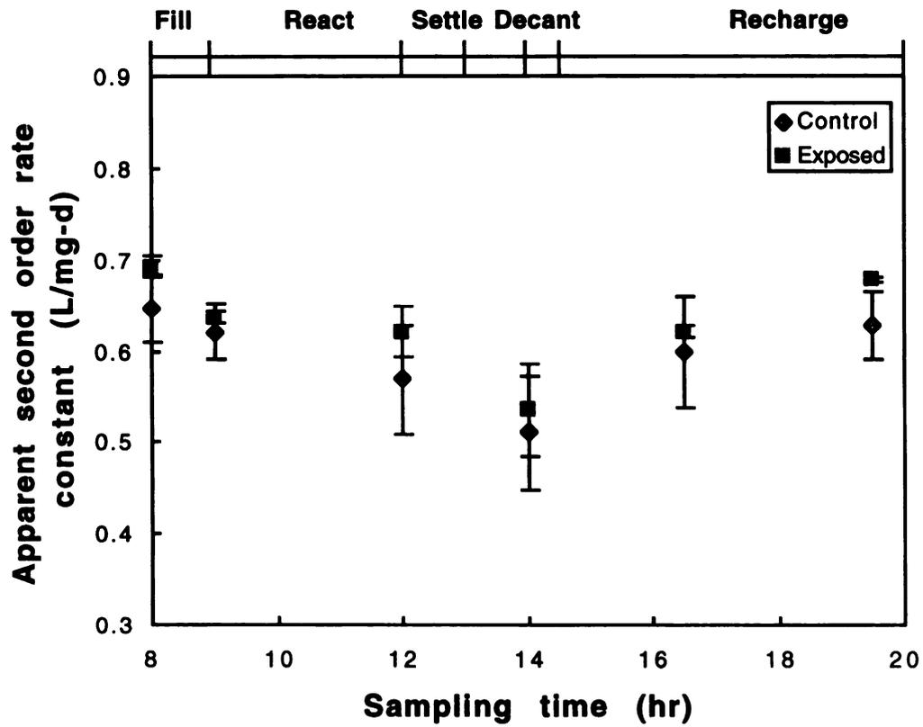
Figure 7.8 Change in the second order rate coefficient for TCE transformation in a typical SBR operating cycle.
