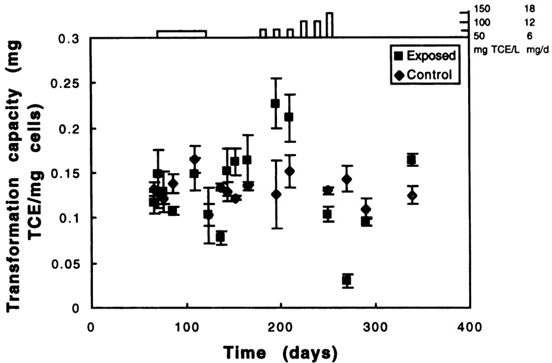
Figure 6.5 Transformation capacity for methanotrophic mixed cultures during long-term TCE exposure
