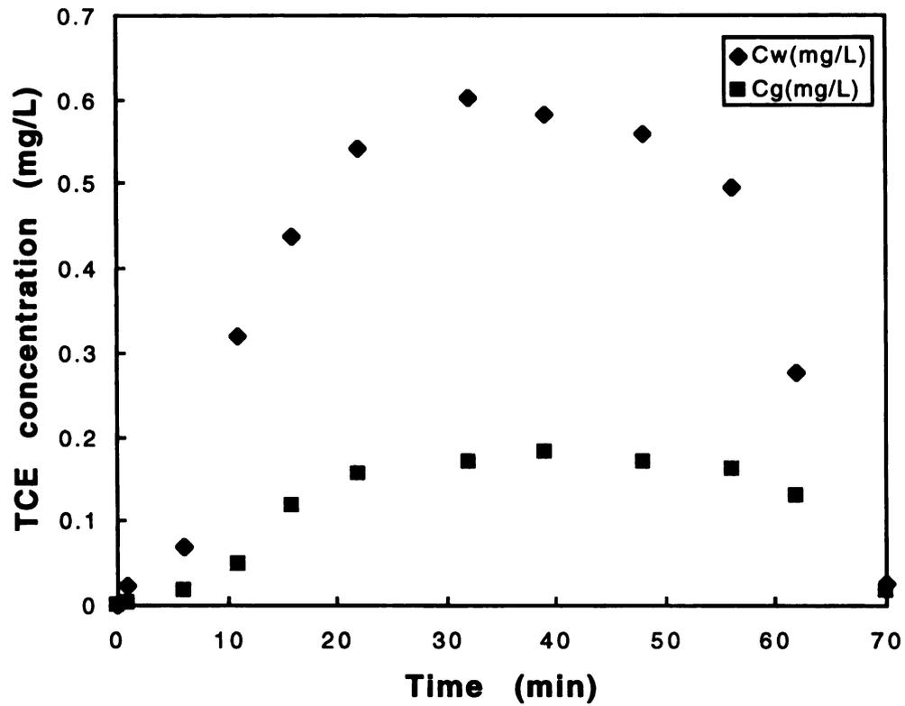
Figure 7.9 TCE concentration in gas ( $C_g$ ) and liquid ( $C_w$ ) phase during the fill and react periods for a feed solution of 25 mg/L TCE.
