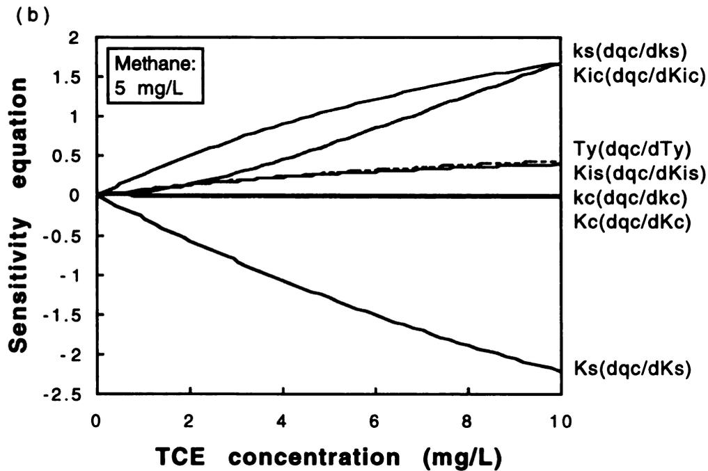
Figure. 5.8 Sensitivity equation for  $q_c$  as a function of TCE concentration for methanotrophic mixed culture at a specified methane concentration.
