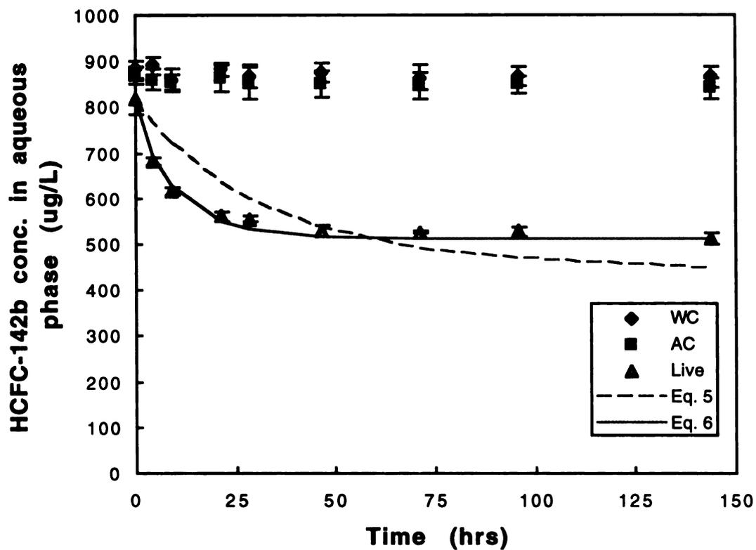
Figure 3.2 Biotransformation of HCFC-142b by methanotrophic mixed culture MM1: model fit based on equation 5 and 6, respectively. Fitting parameters are summarized in Tables 3.4 and 3.5. Error bars give standard deviations for three samples. WC = water control (no cells), AC = autoclaved control, LIVE = 275 mg/L MM1.
