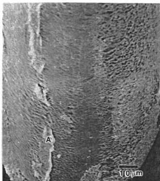
Figure 53 A SEM micrograph of a Ti-coated fiber thermally cycled 150 times.
