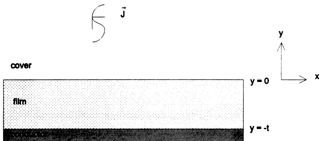
Figure 4.2: Typical background environment in a microstrip circuit.
