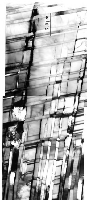
Figure 5.3 - Cross twinning configuration within a large equiaxed \gamma grain.
