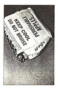
Figure 10: Damaged Apple Package B after Vibration Test 3
