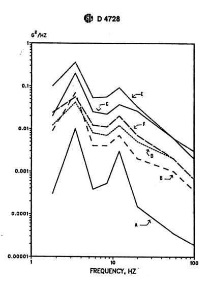
Figure 7: ASTM D4728 X1.2 Power Density Spectrum (Expressway)
