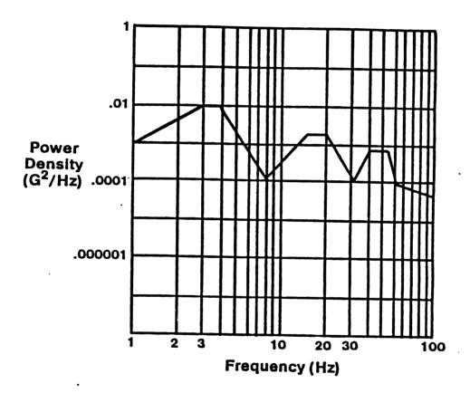
Figure 8: Power Density Spectrum of Leaf Spring Truck
