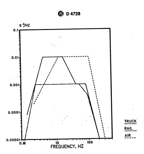
Figure 6: ASTM D4728 X1.1 Power Density Spectrum (Truck)
