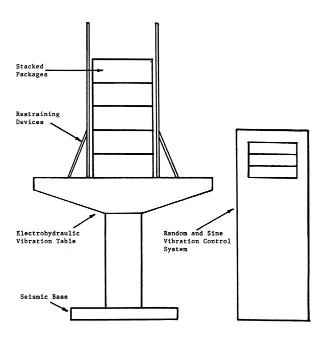
Figure 5: Experimental Test Setup
