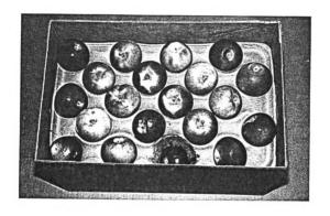
Figure 11: Damaged Apple Package C after Vibration Test 3
