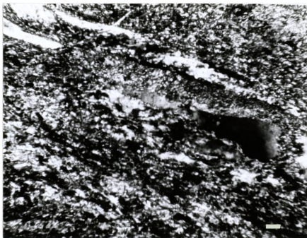
Figure 17. Mylonitized quartz in phyllosilicate rich area. Crossed polars. Scale bar = 100 \mu .
