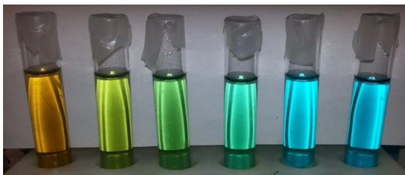
Figure 5-4: Color changes of Q.B. solution in response to concentration of acetol. From left
