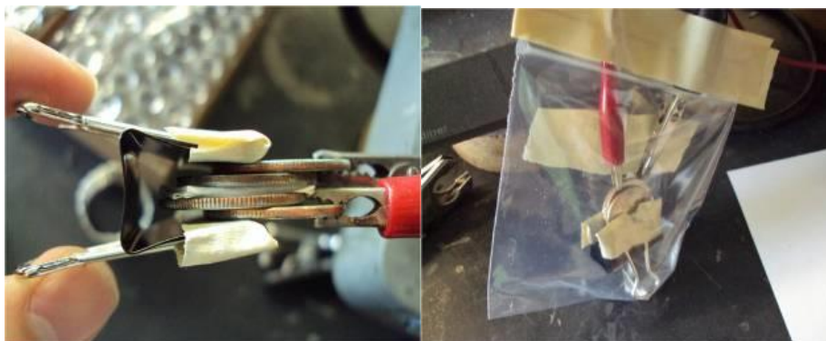
Figure 5-2: (left) Experimental setup of ECH of acetol with coins. A copper coin anode is clipped with red wire, and the nickel coin cathode is clipped with the black wire. An extra coin is added on each side to act as a current collector and provide enough pressure for the clamp (right). Setup is in a small sample bag to prevent filter paper drying.
