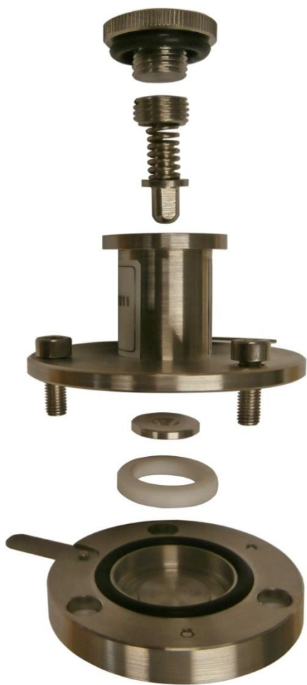
Figure 1-4. Actual coin cell setup used for all electrochemical measurements performed and described in this thesis. These split cells were purchased from MTI-XTL.
