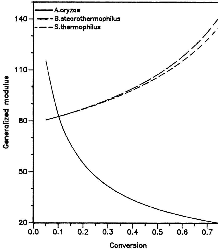
Figure 35. Generalized modulus versus conversion for A.oryzae and bacterial lactases.
