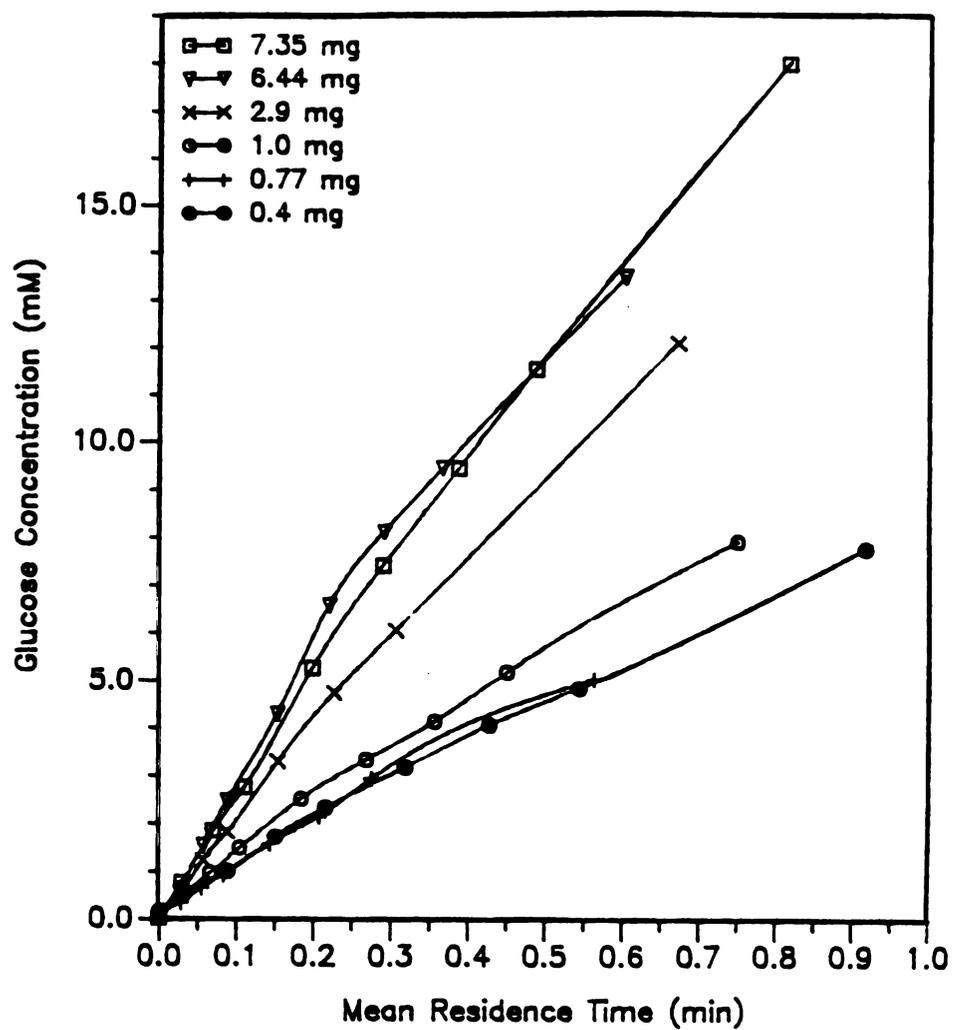
Figure 31. Conversion versus time at various enzyme loadings in a SFR.
