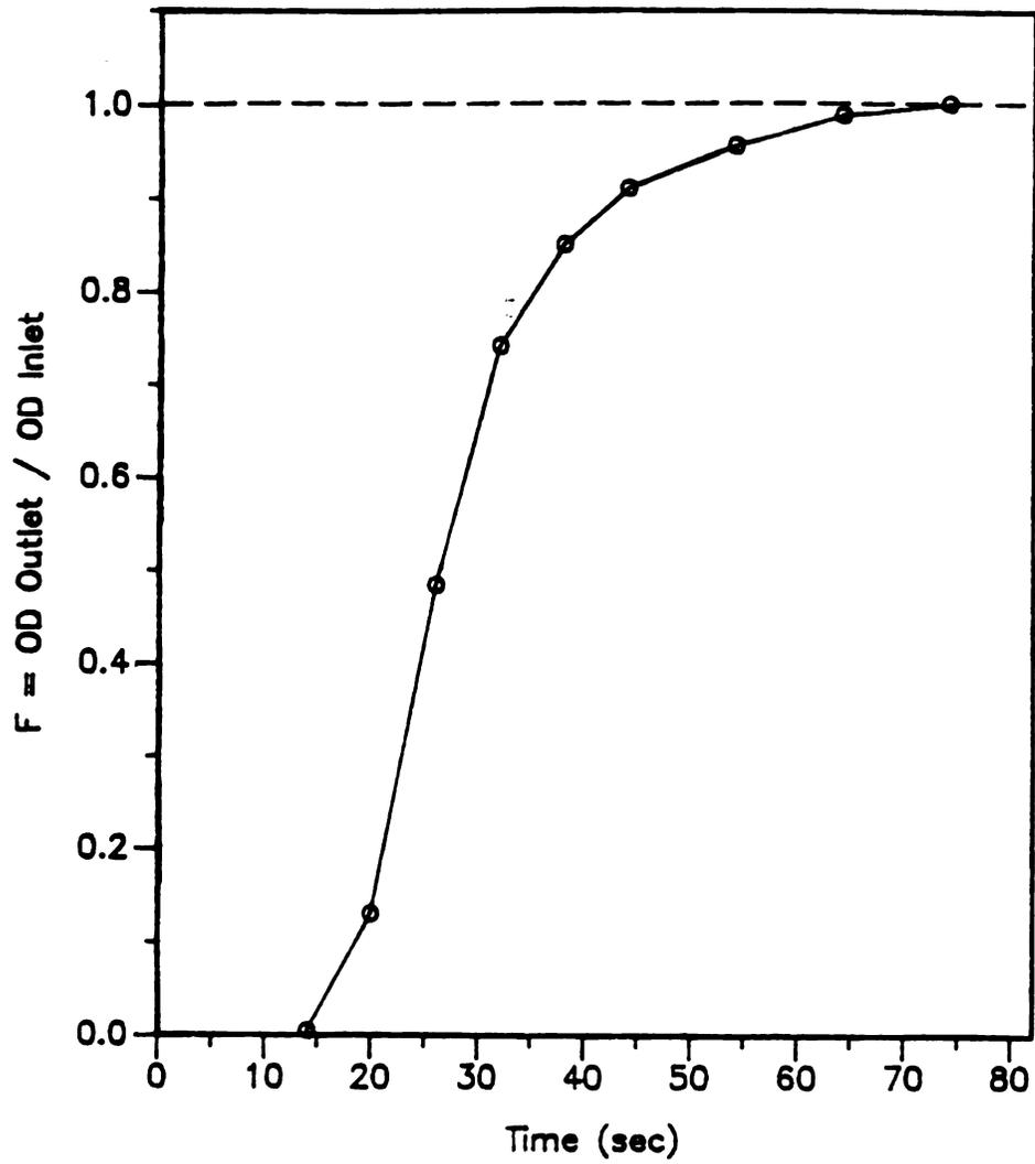
Figure 22. F distribution following step input of blue dextran at flow rate of 99.2 ml/min.
