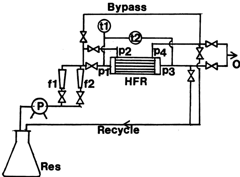
Figure 18. Laboratory hollow fiber reactor system.
