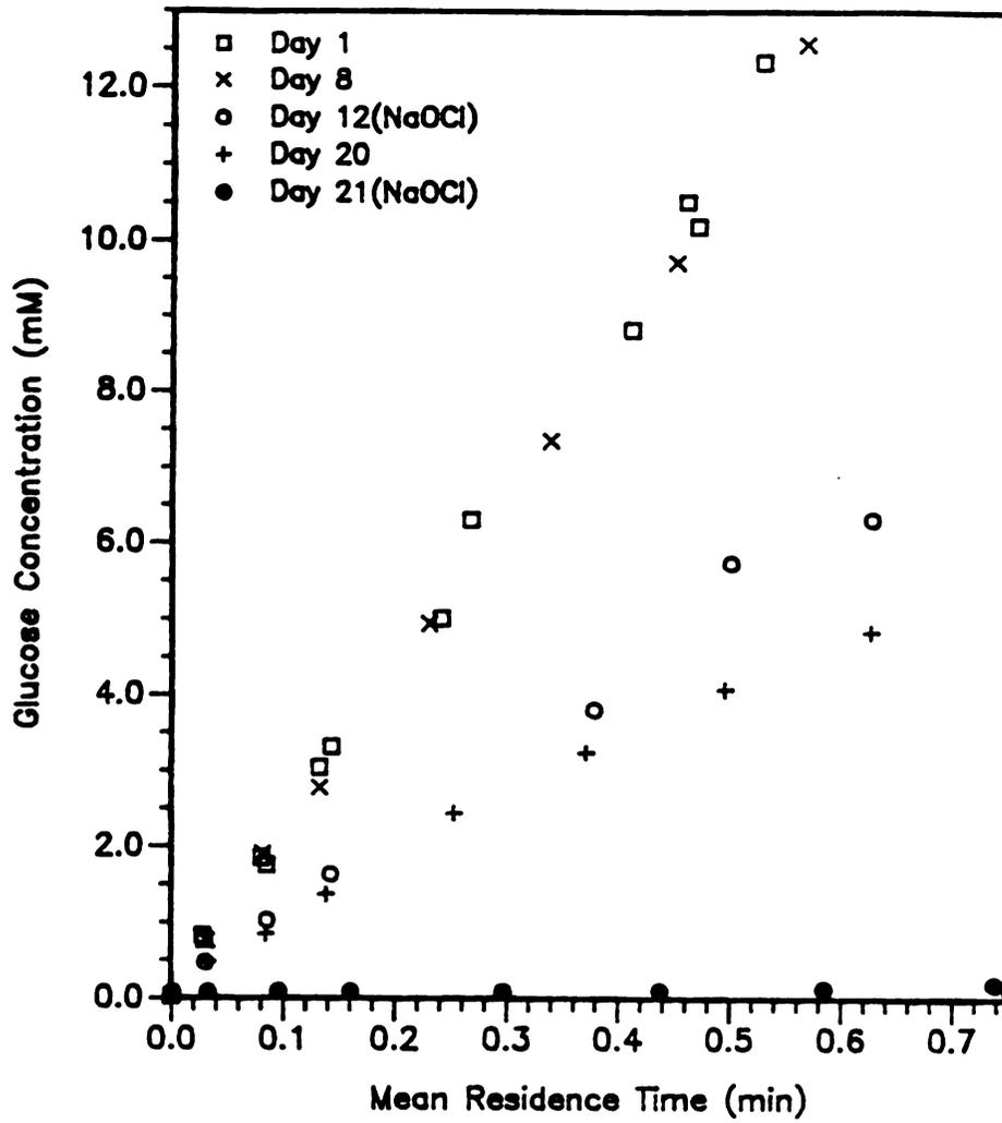
Figure 34. Product concentration in hollow fiber reactor system following storage and treatment with sodium hypochlorite (200 ppm).
