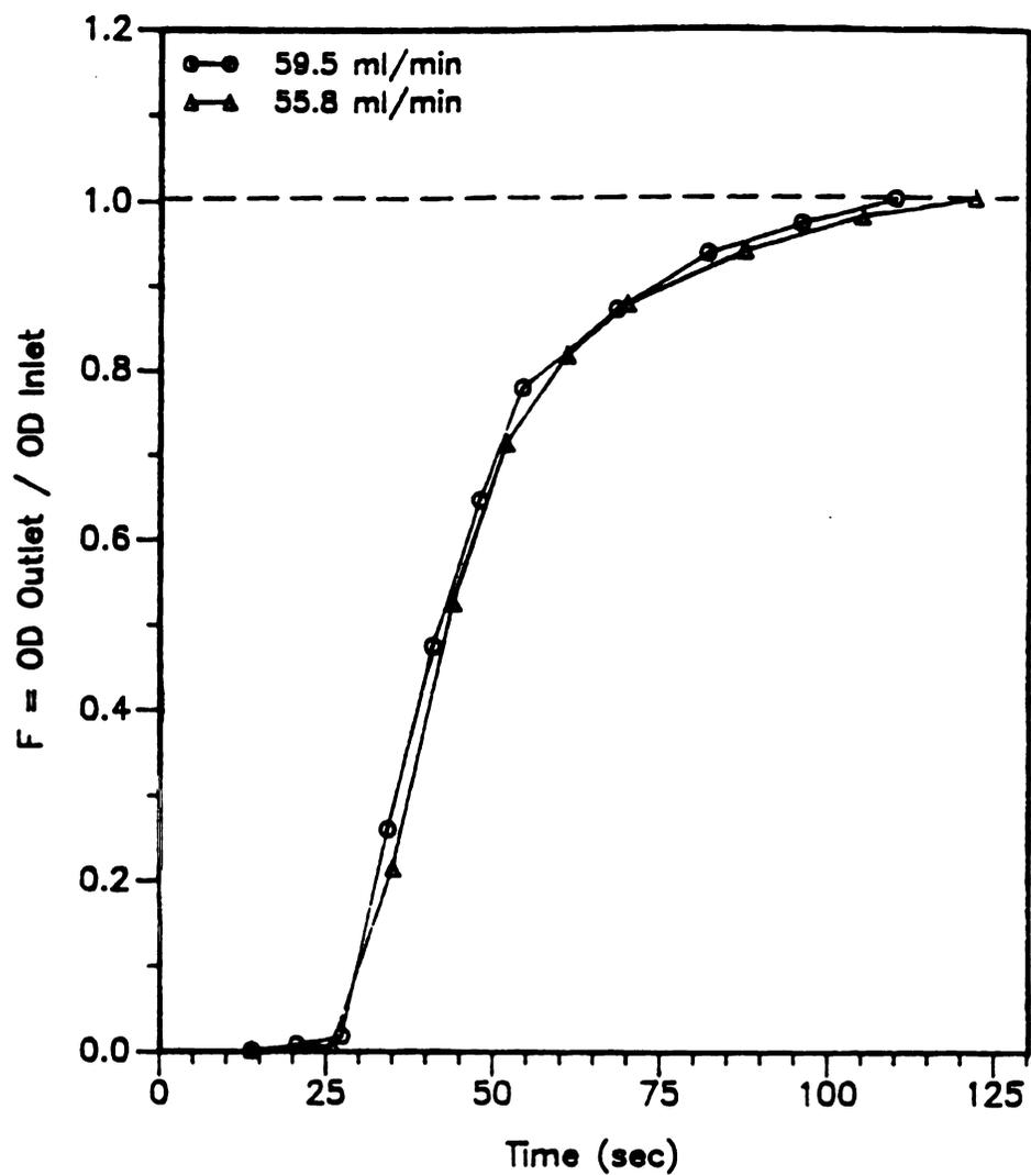
Figure 21. F distribution following step input of blue dextran at flow rate of approximately 55 ml/min.
