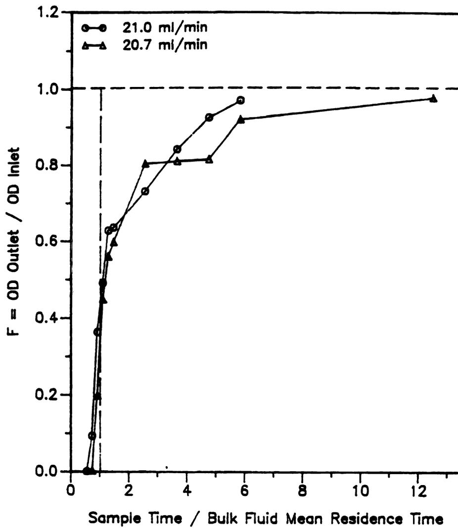
Figure 23. F distribution following step input of lactose at flow rate of approximately 20 ml/min.
