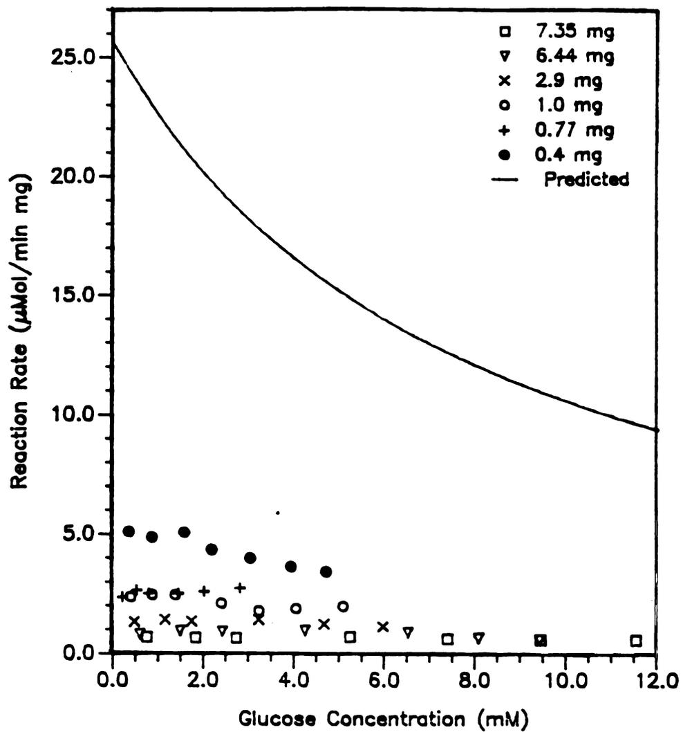
Figure 32. Reaction rate (apparent enzyme specific activity) versus product concentration at various enzyme loadings in a SFR.
