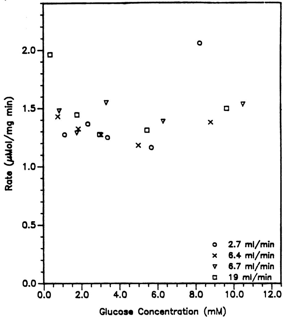
Figure 30. Rate of reaction versus product concentration at three different flow rates in a SFR.
