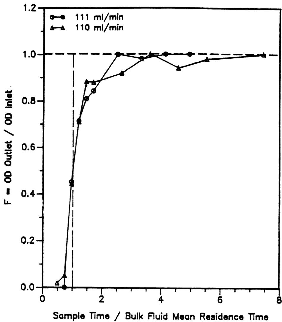
Figure 26. F distribution following step input of lactose at flow rate of approximately 110 ml/min.
