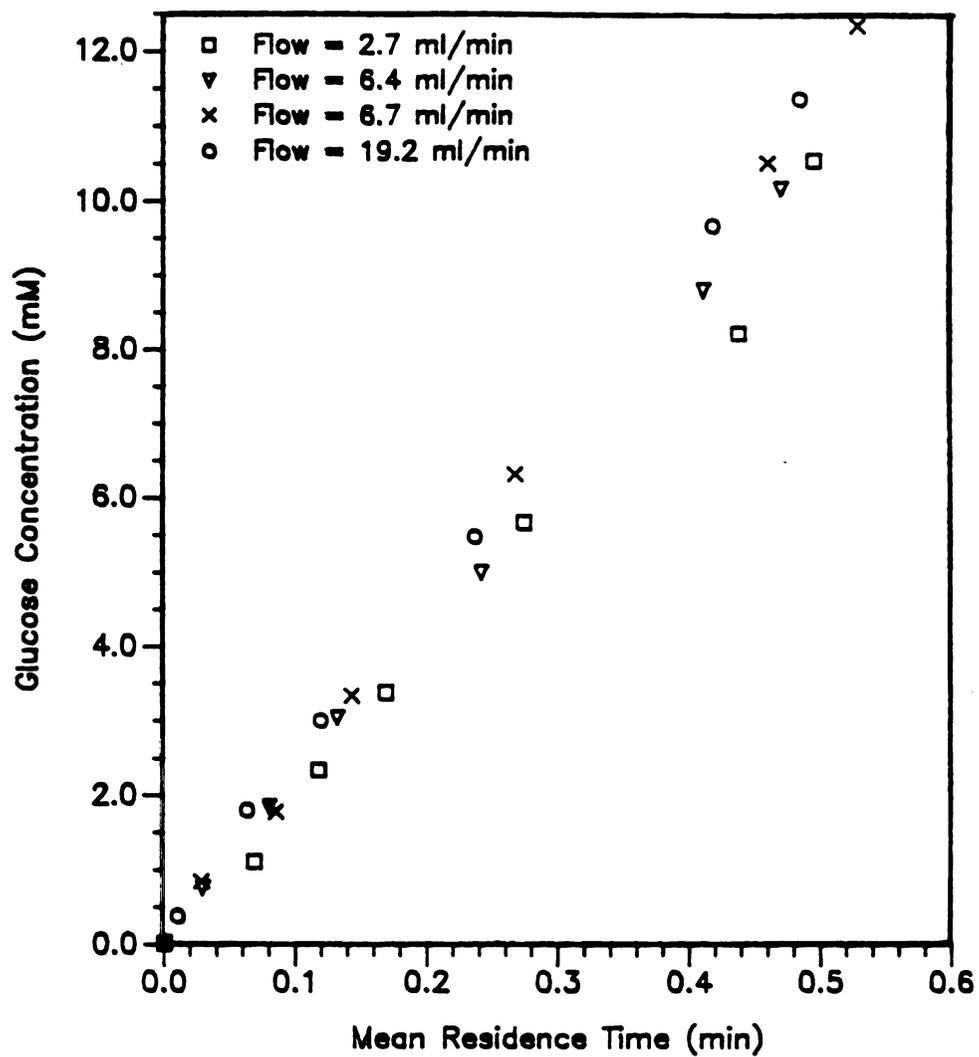
Figure 29. Effect of varying flow rate on conversion in a SFR.
