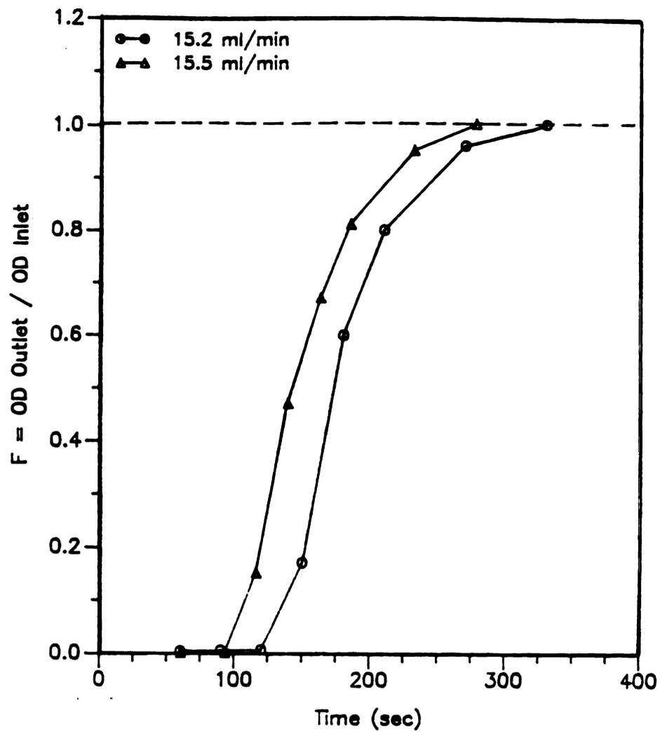
Figure 19. F distribution following step input of blue dextran at flow rate of approximately 15 ml/min.
