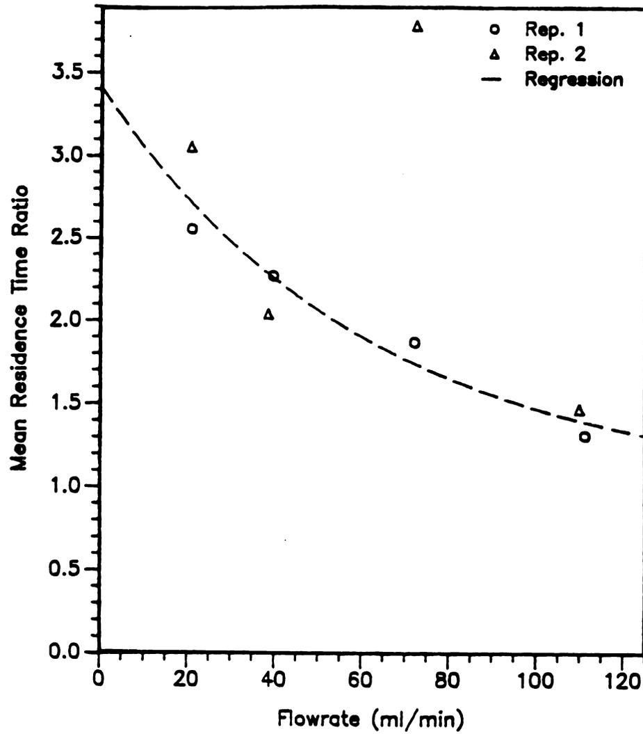
Figure 27. Ratio of lactose mean residence time in hollow fiber cartridge to bulk fluid mean residence time versus flow rate.
