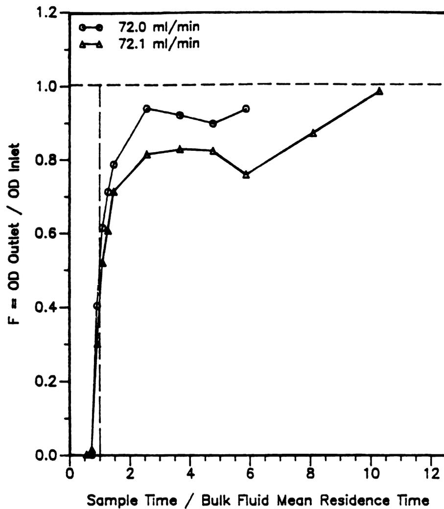
Figure 25. F distribution following step input of lactose at flow rate of approximately 72 ml/min.
