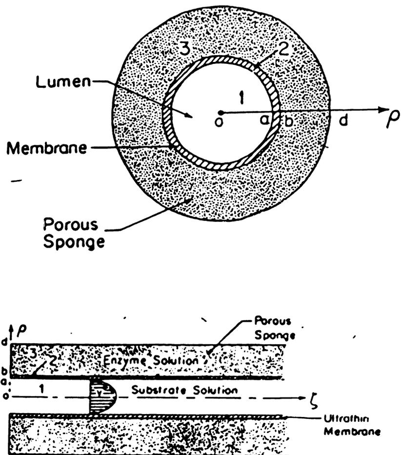
Figure 3. Cross sectional and axial schematics of the regions used in modelling hollow fiber reactors. (Waterland et al. 1974)
