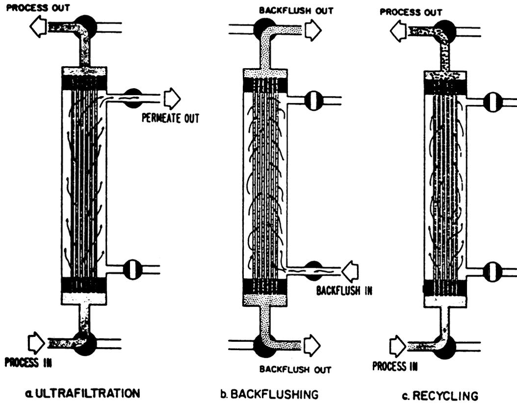
Figure 2. Schematic of hollow fiber cartridge showing the three modes of operation used in system's design. (Breslau and Kilcullen 1978)
