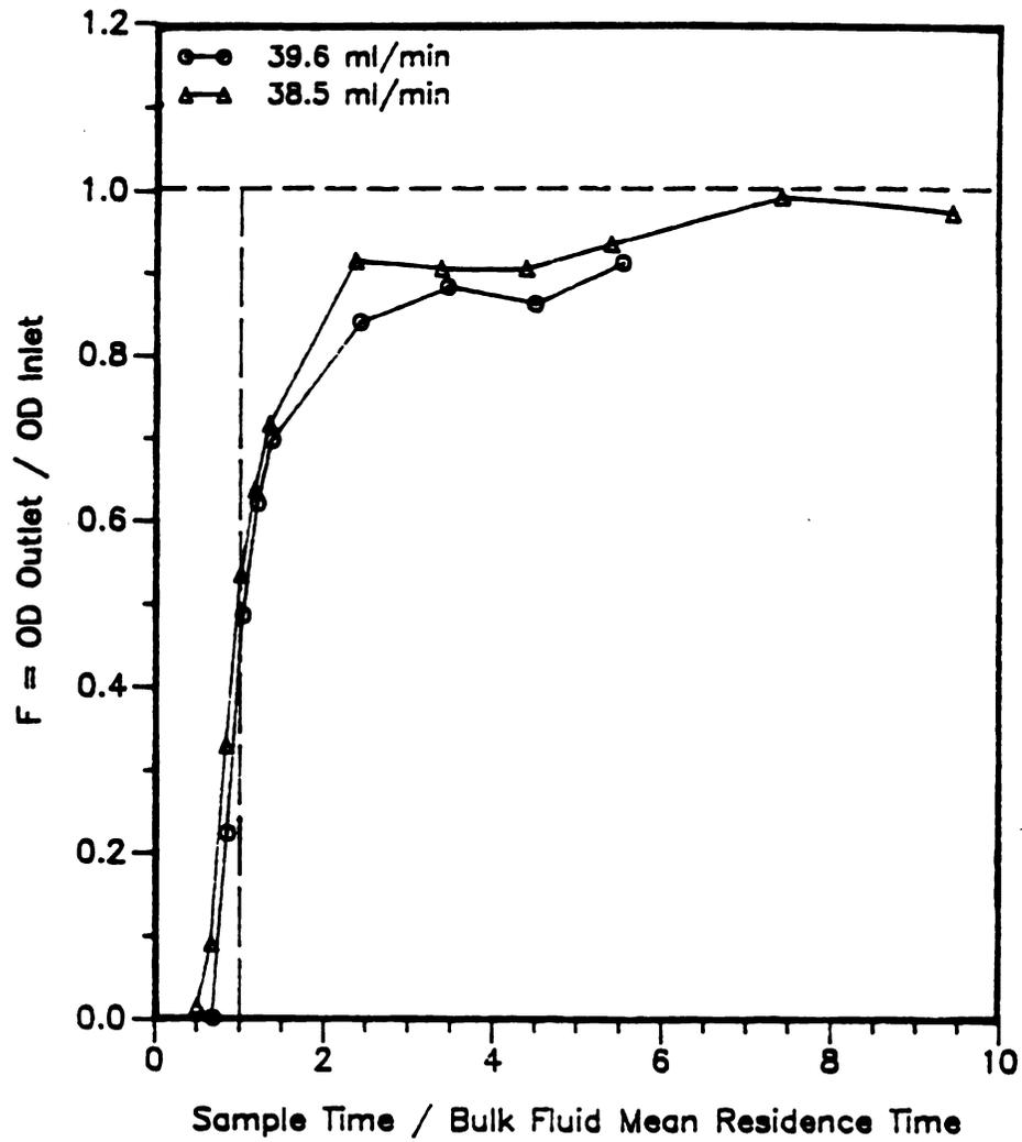
Figure 24. F distribution following step input of lactose at flow rate of approximately 40 ml/min.
