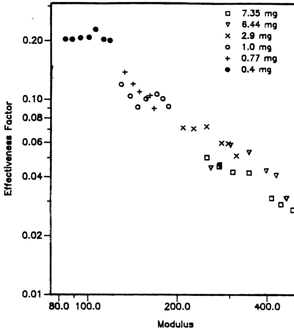
Figure 33. Generalized modulus versus effectiveness factor at different enzyme loadings.
