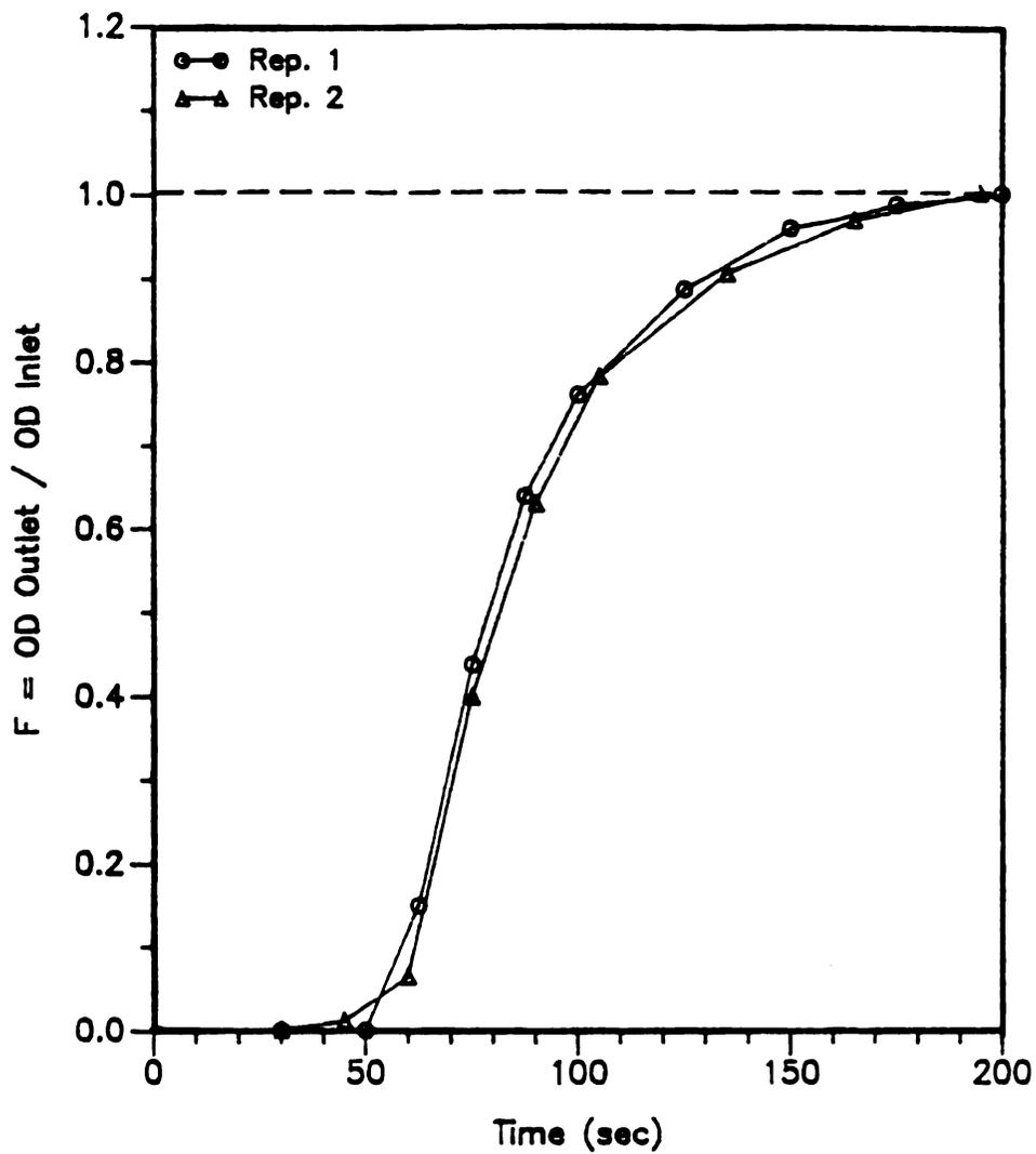
Figure 20. F distribution following step input of blue dextran at flow rate of approximately 32 ml/min.
