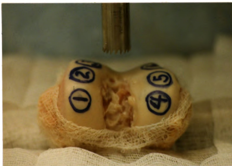
FIGURE 4. Distal femur showing site locations, and set up for hole saw with 1.4 cm bit.
