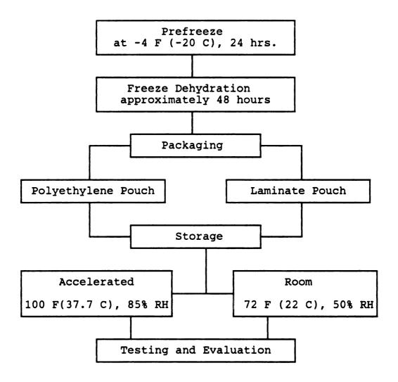
FIGURE 4: Flow Diagram for Yogurt Dehydration and Packaging.
