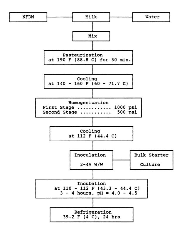
FIGURE 3: Flow Diagram for Yogurt Preparation.
