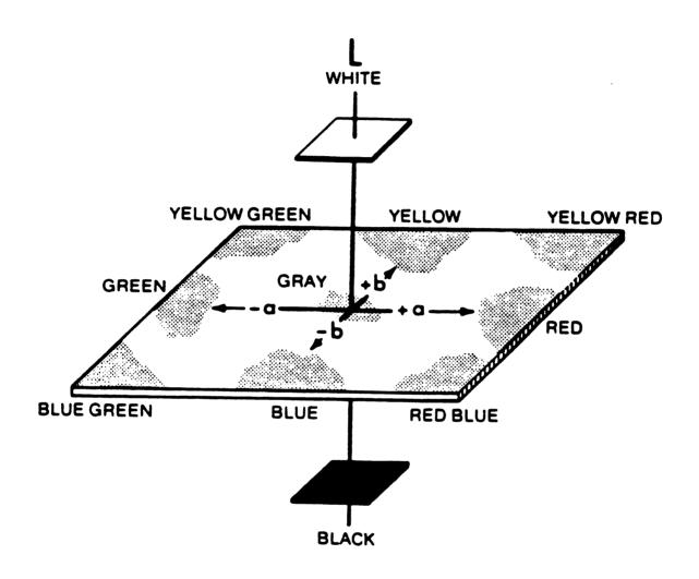
FIGURE 2: L a b System for Color Description and Qualification.
