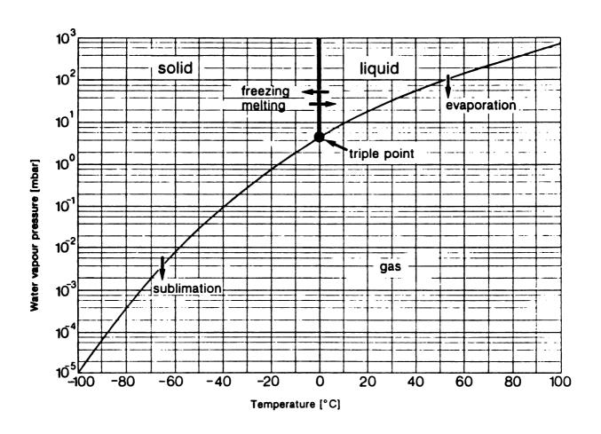
FIGURE 1: Phase Diagram for Water
