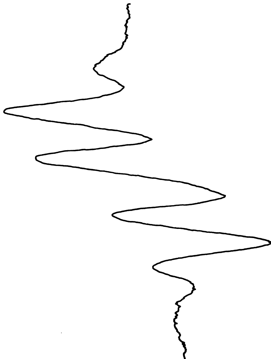
Figure 13. The first-derivative X-band ESR spectrum of -\dot{\text{C}}\text{HCH}_3 in (\text{N}(\text{C}_2\text{H}_5)_4)_2\text{Pt}_2\text{Br}_6 at 77^\circ\text{K} .
