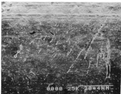
Figure 67. Splashed quenched droplets radiating away from the large surface discontinuity in Figure 65. SEM 150X
