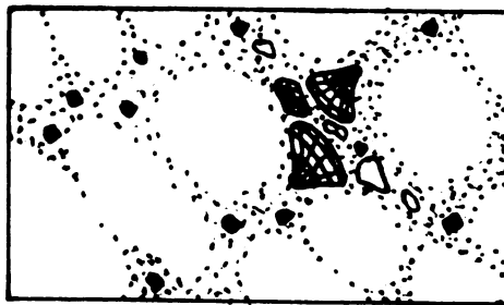
Figure 3. Proposed solidification sequence illustrating segregation associated with solidification (26).
