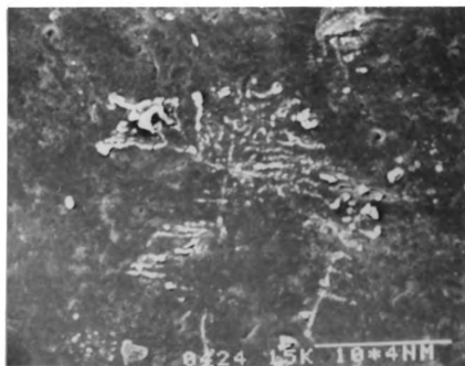
Figure 37. Oxide polyps with a script-morphology. RSEM 300X
