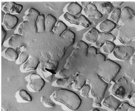
Figure 29. Gamma prime coarsening. RTEM 29,000X
