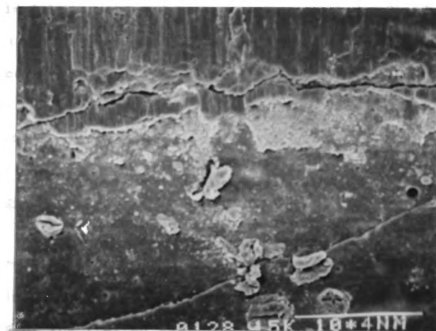
Figure 39. Crack of Specimen F109-1 F developed between cycles 31,587 and 46,587, this crack runs near the fretted slip/no-slip boundary and also extends into the notched region. RSEM 150X, 300X
