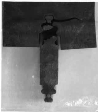
Figure 15. Specimen F109-10 Cr, A end, loading grip #3. 1.55X
