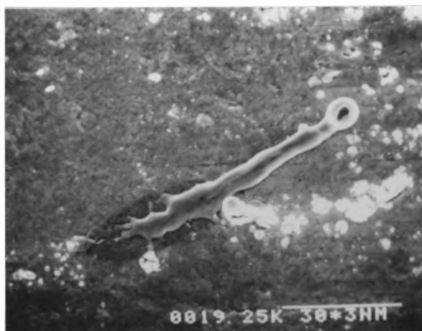
Figure 61. Incipient melting splashed sphere on F109-5 F, similar to those in figure 60. SEM 1000X
