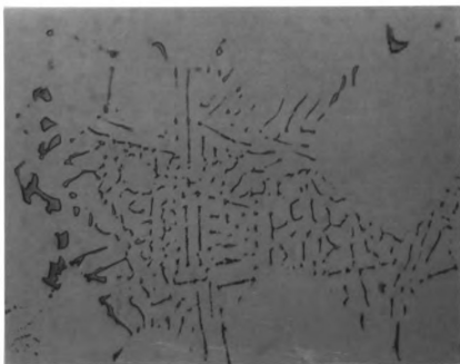
Figure 24. Chinese-script (rosette) MC-type carbides. OM 400X
