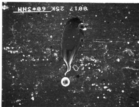
Figure 62. Dripping sphere: incipient melting area characterized by glassy, very smooth appearance. SEM 500X
