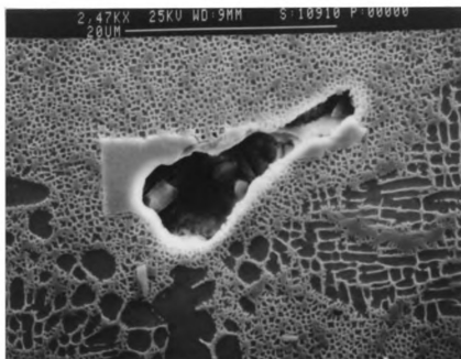
Figure 27. A micropore associated with a carbide. SEM 2,470X
