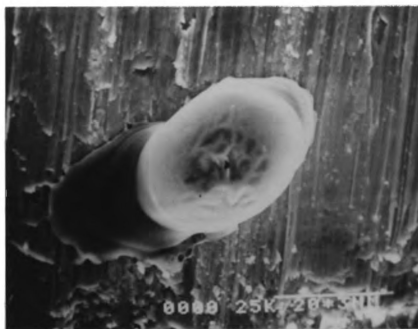
Figure 64. A spherical particle located just inside the boundary of the wear region where localized melting has occurred and recorded the cyclic movement in the smooth melted region. SEM 1500X
