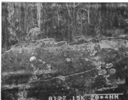
Figure 39. Crack of Specimen F109-1 F developed between cycles 31,587 and 46,587, this crack runs near the fretted slip/no-slip boundary and also extends into the notched region. RSEM 150X, 300X
