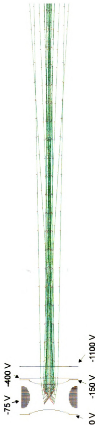
Figure 2-20. Trajectories of ions extracted from a quadrupole ion trap. The green lines are the ion trajectories. The red dots are ion positions along the flight path at 0.5 \mu s intervals. The m/z 100 ions are initially placed in the segmented ring ion trap source in an X pattern. The voltages applied to the electrodes are indicated.
