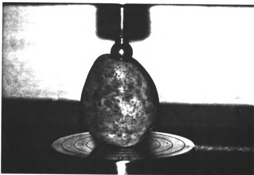
Figure 5.1 Bruising a potato at the stem end using a (7/8 inch dia) spherical indenter on an Instron Testing machine.
