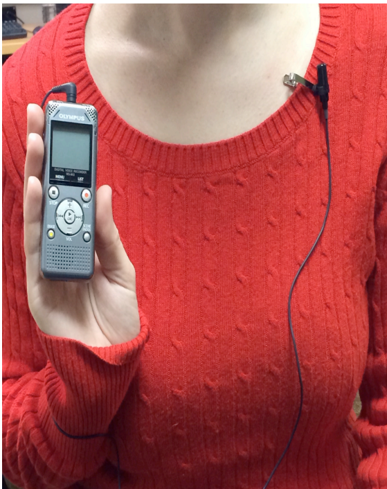
Figure 2: Female talker wearing the tie clip microphone plugged into the digital recorder.
