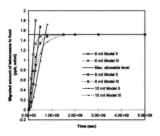
Figure 12 The migration profile of tetracosane for a lamination of 1.15 mil contaminated HDPE layer/ 6, 8, 10 mil HDPE barrier layer by Models II and III
