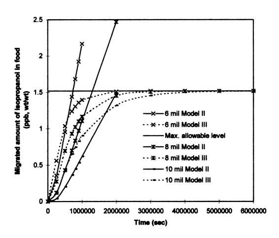
Figure 10 The migration profile of isopropanol for a lamination of 1.15 mil contaminated HDPE layer/ 6,8,10 mil HDPE barrier layer by Models II and III
