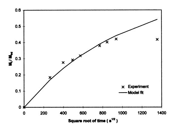
Figure 25 The profile of the comparison of migration of tetracosane between the experiment and the model fit for sample 6
