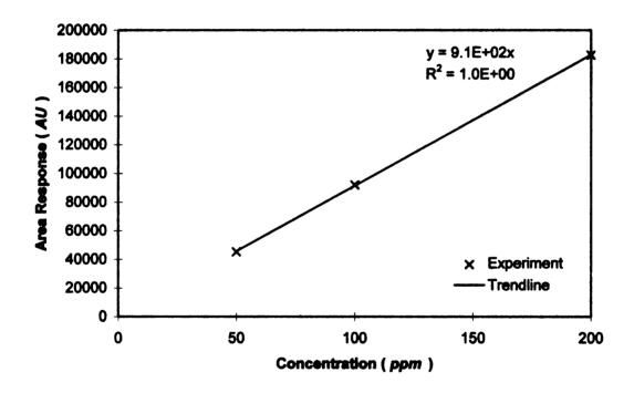
Figure 18 Standard calibration curve of isopropanol for HP 6890 by SPME
