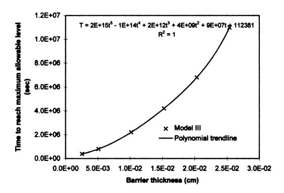
Figure 13 The relation of time to reach maximum allowable level as a function of a barrier thickness for isopropanol as initial concentration of 0.84ppm
