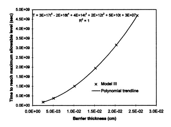
Figure 14 The relation of time to reach maximum allowable level a function of a barrier thickness for tetracosane as initial concentration of 0.84ppm
