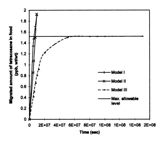
Figure 6 The profiles of the migrated amount of tetracosane from a single layer and a laminated film based on predictive Models I, II and III
