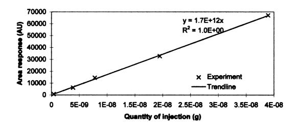
Figure 19 Standard calibration curve of hexane for HP 5890A
