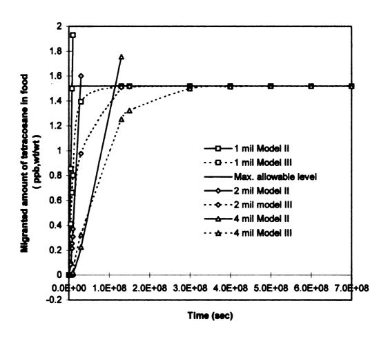
Figure 11 The migration profile of tetracosane for a lamination of 1.15 mil contaminated HDPE layer/ 1, 2, 4 mil HDPE barrier layer by Models II and III
