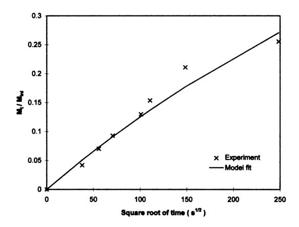
Figure 20 The profile of the comparison of migration of tetracosane between the experiment and the model fit for sample 1
