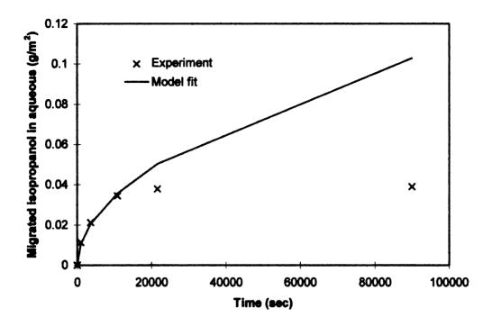
Figure 4 Migrated amount of Isopropanol from spiked HDPE film into aqueous phase (water) at 23 °C
