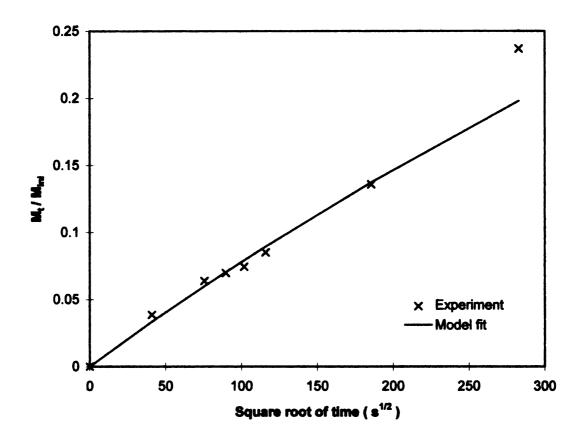
Figure 21 The profile of the comparison of migration of tetracosane between the experiment and the model fit for sample 2
