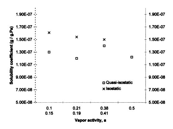
Figure 3 Solubility coefficient of Isopropanol in HDPE film at 23 °C by Quasi-isostatic and Isostatic permeation techniques.
