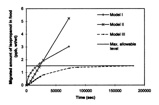
Figure 5 The profiles of the migrated amount of isopropanol from a single layer and a laminated film based on predictive Models I, II and III
