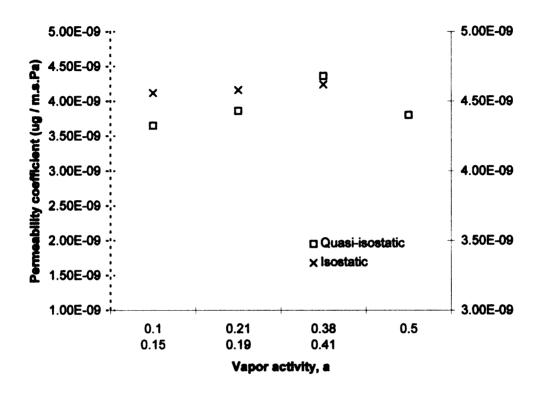
Figure 2 Permeability coefficient of Isopropanol through HDPE film at 23 °C by Quasi-isostatic and Isostatic permeation techniques.
