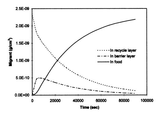
Figure 7 The migration profile of isopropanol for a lamination of 1.15 mil contaminated HDPE layer/1 mil HDPE barrier layer by Model III
