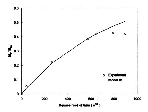
Figure 23 The profile of the comparison of migration of tetracosane between the experiment and the model fit for sample 4
