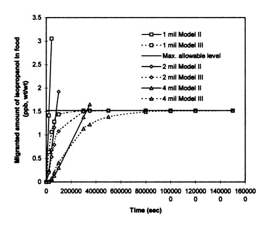
Figure 9 The migration profile of isopropanol for a lamination of 1.15 mil contaminated HDPE layer/1, 2, 4 mil HDPE barrier layer by Models II and III
