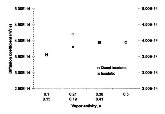
Figure 1 Diffusion coefficient of Isopropanol in HDPE film at 23 °C by Quasi-isostatic and Isostatic permeation techniques.
