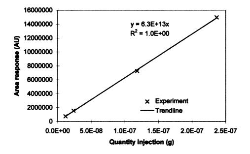
Figure 17 Standard calibration curve of isopropanol for GC-MS
