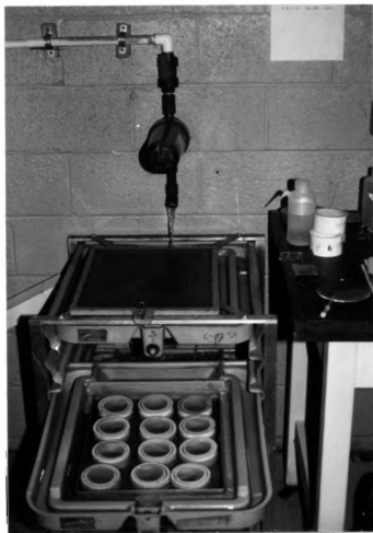
Figure 4. Photograph of heath incubation unit used to incubate bluegill embryos and fry.
