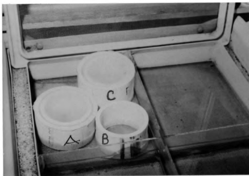
Figure 1. Photograph of two part PVC bluegill incubation chambers, placed in heath incubator unit. (A = top chamber, B = bottom chamber, C = top chamber over bottom chamber).
