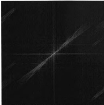
Figure 25. Test FFT image for calibration of braid angle analysis.
