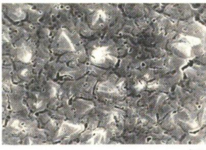
Figure 7.5: Planarized surface after processing with high  $O_2$  containing plasmas
