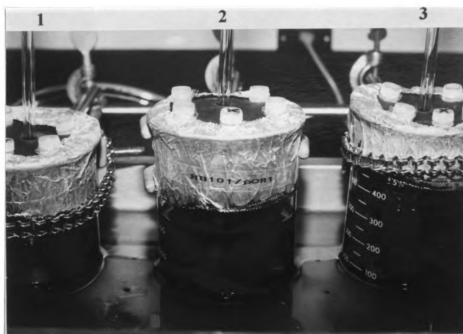
Figure 24. Removal of selenite from LB broth. Each strain, S. maltophilia ORO2 (1), MJ800 (2), and HB101 (3), was grown overnight in 250 ml of LB broth, pelleted and resuspended in 40 ml of LB broth. Samples of 10 ml were added to dialysis bags immersed in LB broth containing 10 mM selenite.
