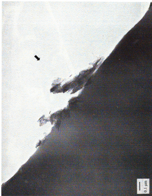
Figure 4.25 Transmission electron micrograph of an ultramicrotomed section obtained from the strained dog-bone coupon of 200 °C treated coated fiber showing the coating adhering to the matrix. The direction of the knife is shown by the arrow.
