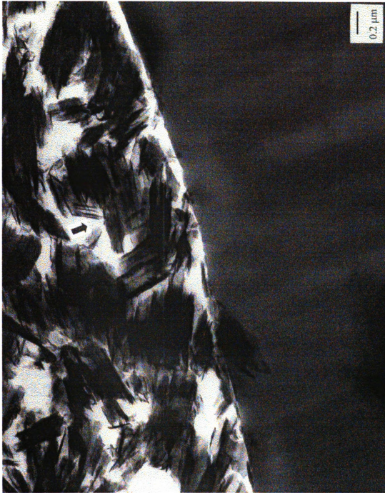
Figure 4.26 Transmission electron micrograph of an ultramicrotomed section obtained from the strained dog-bone coupon of 800 °C treated coated fiber showing the coating adhering to the matrix. The direction of the knife is shown by the arrow.
