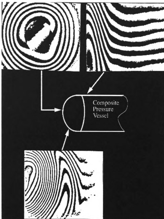
Fig. 5.42 Out-of-plane displacement contour maps around a fiber over-wrapped composite vessel.
