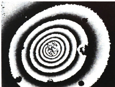
Fig. 5.43 Out-of-plane displacement contour created by fastening a screw into a honeycomb table.
