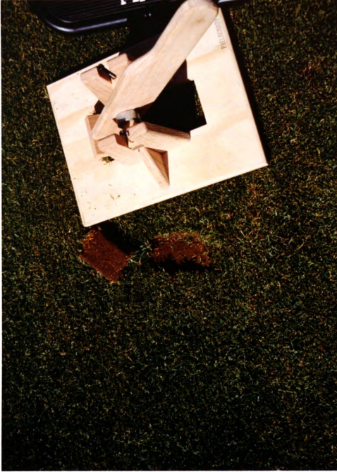
Figure 1: Radial Sod Extraction Device (Divot Cutter)
