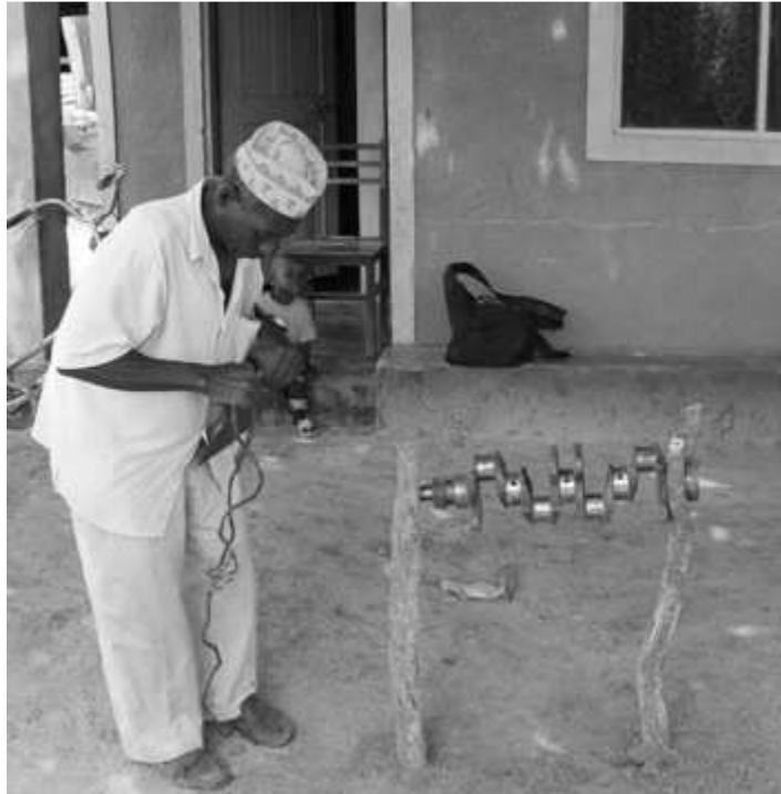
Figure 1.11: Jumanne Mrisho demonstrating the manual repair of crank shafts in Tabora. Photograph by author.
