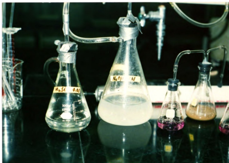
Figure 2.1. The inflowing air was cleaned by passing it through 0.1N NaOH and 0.01N H 2 SO 4 .
