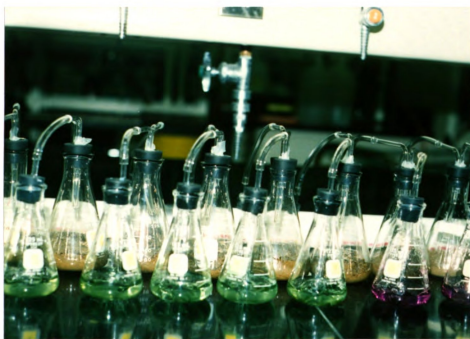
Figure 2.2. The clean air was directed through the Erlenmeyer flask containing soil and through 40 ml of 5% boric acid solution to trap NH 3 .
