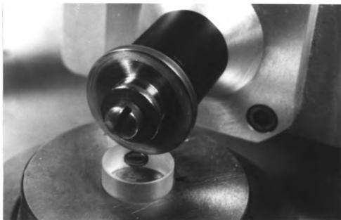
Figure 2.11 Dimpler wheel and TEM specimen on Pyrex™ stub.
