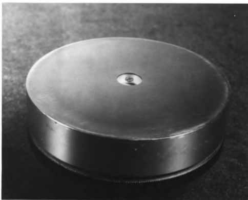
Figure 2.10 Sectioned disc and stub in Gatan™ Disc Grinder.
