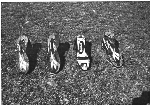
Figure 2. The 4 shoes used for testing friction and traction are, from left to right, a) the Reebok Wet Rat, b) the Dry Rat, c) Viscious, and d) Pit Bull.
