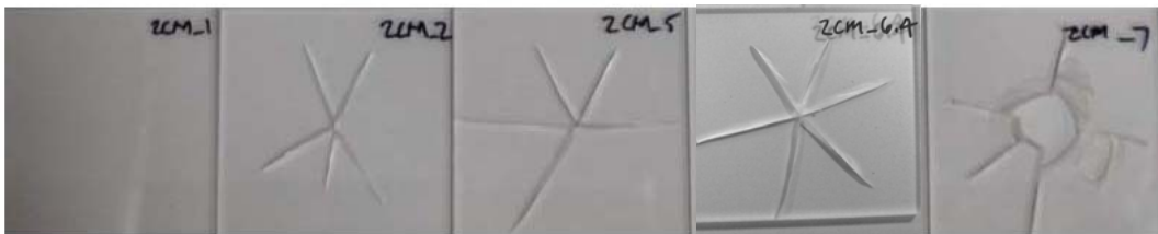
Figure 2.2 Post-failure pictures of mono-PMMA plates under constant impact mass: velocities are 0.7 m/s, 1.0 m/s, 2.0 m/s, and 3.0 m/s respectively from left to right.
