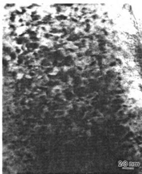
Figure 4.38 High magnification TEM observation on 1 \times 10^{16} \text{ Ar}^+ \text{ cm}^{-2} implanted zone.
