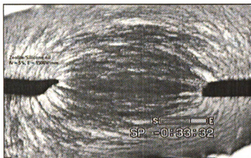
Fig. 1. Chain Structure of Zeolite / Silicone Oil Exposed to Electric Field
