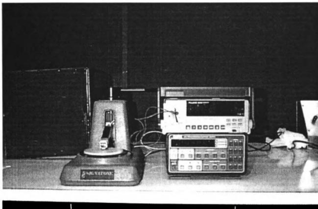
**Figure 5.11 Photograph of the Four Probe instrument**
