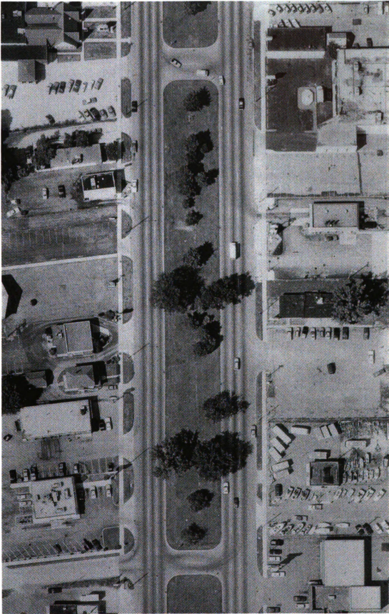
Figure 1.1.5 Urban Boulevard Section With Bidirectional Cross-Over
