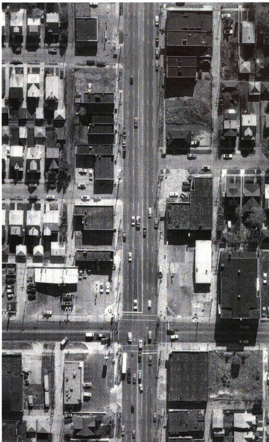
Figure 1.1.8 Urban Seven-Lane Center Left-Turn Lane Cross-section
