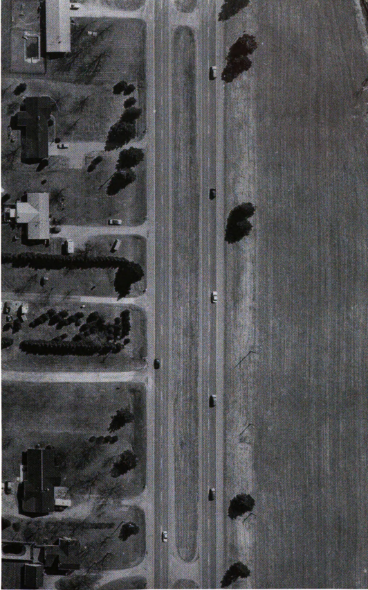
Figure 1.1.3 Rural Boulevard Section With Bidirectional Cross-Over and Residential Drives
