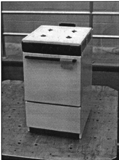
Figure 28 - Sample EV201 on the vibration table
