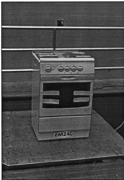
Figure 31 - Sample EM240 on the vibration table
