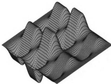
Figure 5.2: The radial component of the magnetic field for the triplet when the currents for the three quadrupoles are 5, 15 and 10 A respectively.
