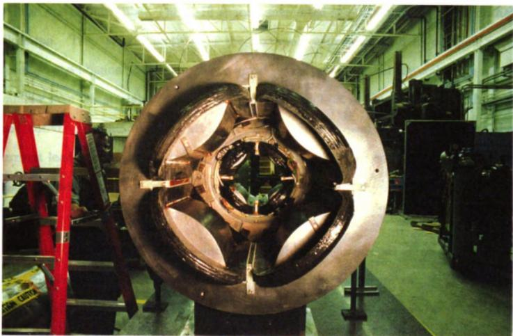
Figure 4.21: Q1 and Q2 coils assembly.
