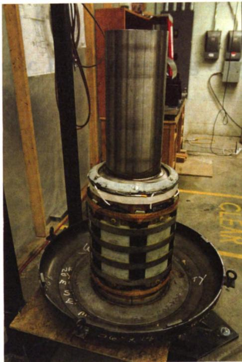
Figure 4.22: Sextupole coils assembly.
