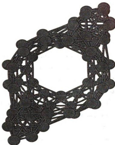
Figure 1.2: A unit cell of L-zeolite (also called cage) showing the main channel viewed along the channel axis. Only oxygen atoms of the framework are shown.
