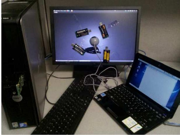
Figure 3.3 Testbed for light spot detection. 4 TelosB motes and a webcam detect the light spot. For interpretation of the references to color in this and all other figures, the reader is referred to the electronic version of this dissertation.
