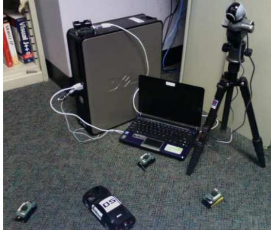
Figure 3.7 Testbed for acoustic target detection. 3 Iris motes and a webcam detect the moving toy car.
