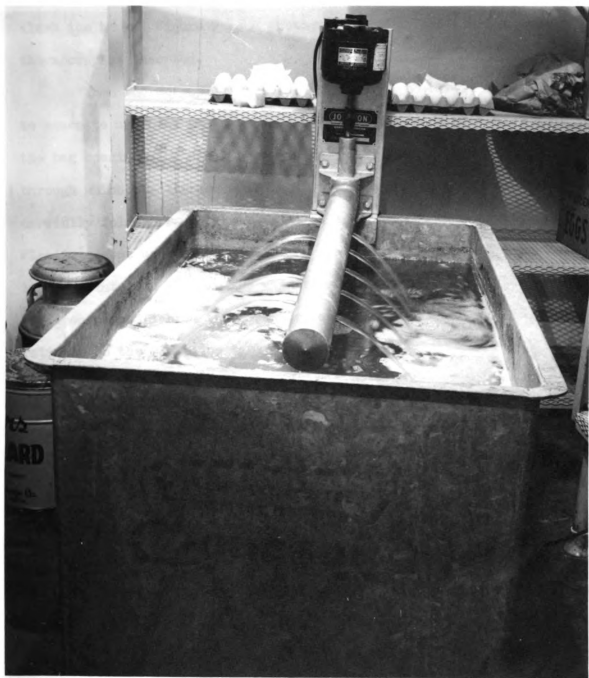
Fig. 6. Photograph of a chill tank containing slush ice and circulating liquid used to maintain constant temperatures of turkeys.
