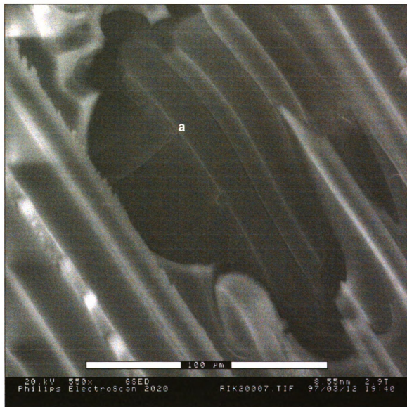
Figure 7.3 ESEM micrograph of a fracture surface after fracture toughness testing (a = pull-out of rubber particle)
