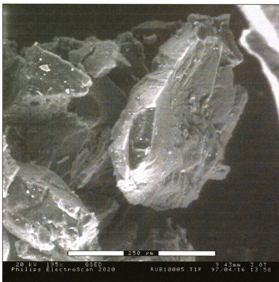
Figure 5.7 ESEM micrograph of untreated rubber particles
