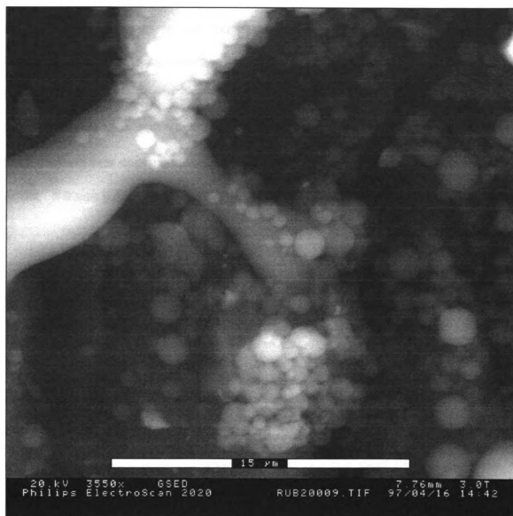
Figure 5.10 ESEM micrograph of rubber binder particles
