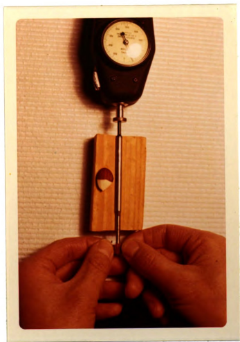
Figure 3. Apparatus for testing seed coat strength.
