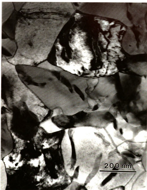
Figure 3-18. TEM BF image taken from the surface of the film H773 showing the coarse grains and precipitates.
