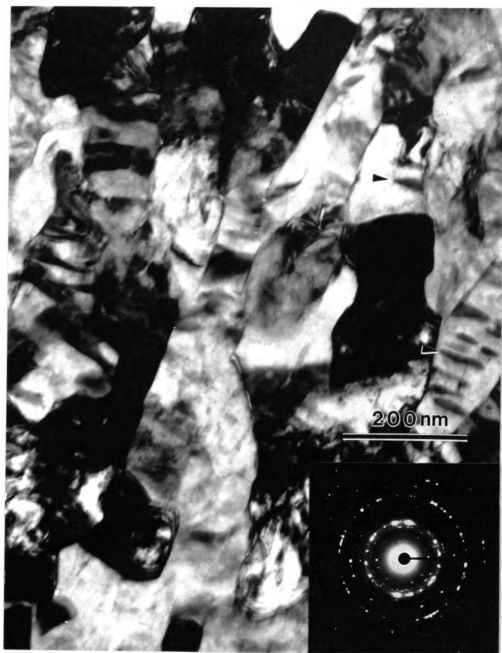
Figure 3-15. The micrograph and associated SADP taken at the midplane of the film H703 revealing crystalline B2 grains and transgranular precipitates (indicated by arrows).
