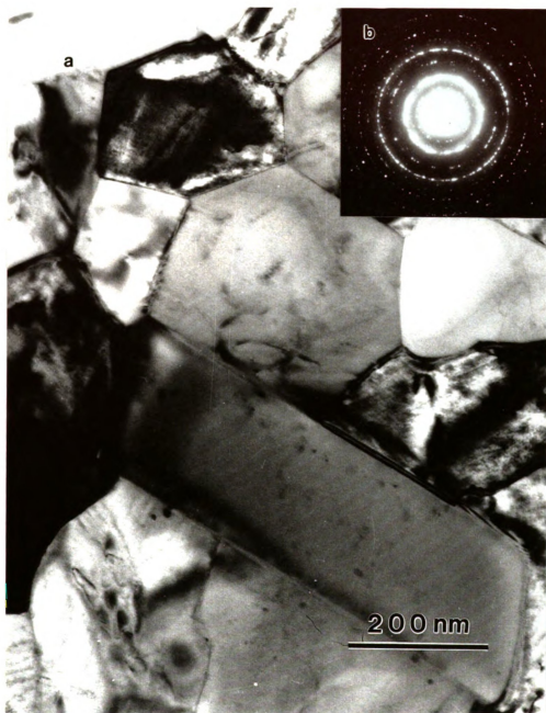
Figure 3-29. TEM bright-field image and SADP of film A3 which was produced by aging the film H723 at 858 K for 1 hour and furnace cooling. The SADP in (b) was taken at 30^\circ tilt showing random grain orientation.
