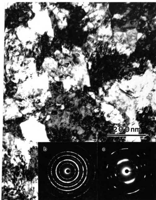
Figure 3-9. TEM BF images and the associated SADP's taken from the midplane of the film H673. The BF image (a) and (d), respectively, were recorded at a tilt of 0 and 45 degrees. A precipitate particle displays a perfect 'butterfly' shape of the image contrast as indicated by the arrow. Again, elongated grain images in (d) implies a columnar grain structure. The SADP (b) and (c) were recorded at a tilt of 0 and 30 degrees, respectively, showing a strong (110) fiber-texture.
