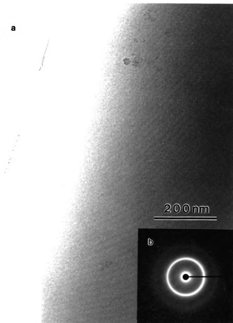
Figure 3-1. TEM bright-field (BF) image in (a) showing a completely featureless structure, and the associated selected area diffraction pattern (SADP) in (b) showing a broad, diffuse halo pattern which are normally observed in the amorphous materials. The micrographs were taken from the midplane of the film H573 at a tilt of 0 degree.
