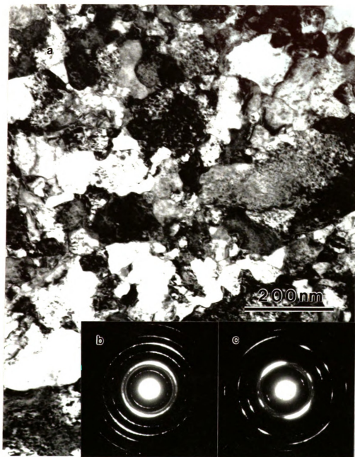
Figure 3-7. TEM BF image and the associated SADP's taken from the surface of the film H623. The SADP (b) and (c) were recorded at a tilt of 0 and 30 degrees, respectively, showing a strong (110) fiber-texture.
