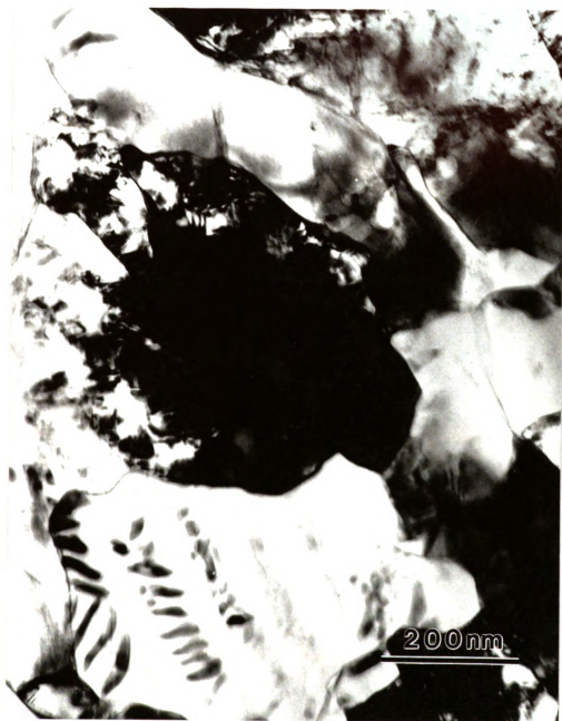
Figure 3-14. TEM BF image taken from the surface of the film H723. The precipitates show smaller size than that in the midplane. Three ranges of precipitates can be seen in the low part of the micrograph.
