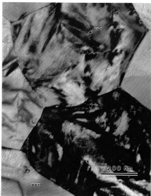
Figure 3-31. TEM image of the film A5 obtained by annealing film H673 at 988 K for 1 hour and furnace cooling. The size of grains have increased during annealing. Obviously, the bulk diffusion for NiTi grain growth have occurred.
