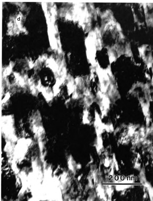
Figure 3-9. (Continued) TEM BF images and the associated SADP's taken from the midplane of the film H673. The BF image (a) and (d), respectively, were recorded at a tilt of 0 and 45 degrees. A precipitate particle displays a perfect 'butterfly' shape of the image contrast as indicated by the arrow. Again, elongated grain images in (d) implies a columnar grain structure. The SADP (b) and (c) were recorded at a tilt of 0 and 30 degrees, respectively, showing a strong (110) fiber-texture.
