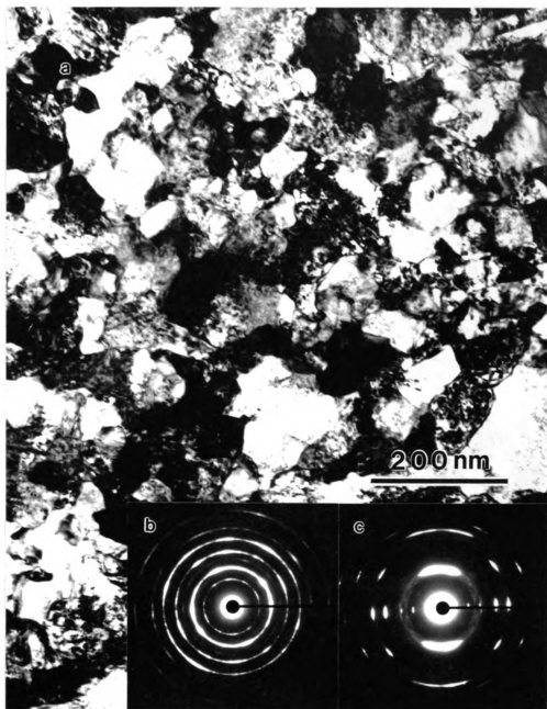
Figure 3-4. TEM BF images and the associated SADP's taken from the surface of the film H598. The BF image (a) and (d), respectively, were recorded at a tilt of 0 and 45 degrees. Elongated grain images in (d) suggests a columnar grain structure. The SADP (b) and (c) were recorded at a tilt of 0 and 30 degrees, respectively, showing a strong (110) fiber-texture. The non-even intensities of the diffraction rings in (b) reflect the restricted in-plane grain orientations.
