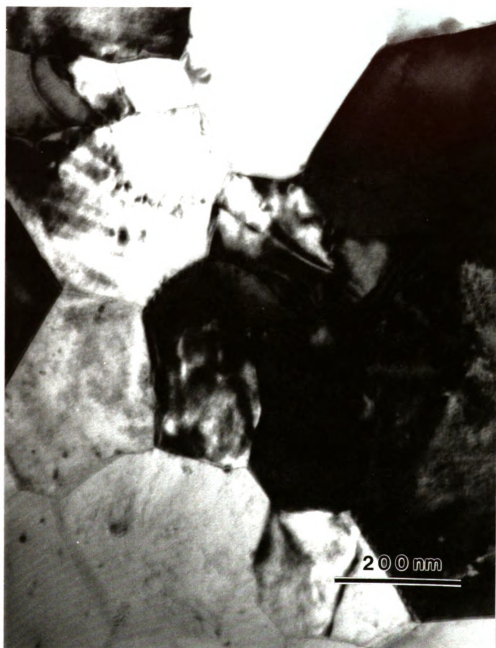
Figure 3-30. TEM bright-field image of film A4 which was produced by aging the film H723 at 813 K for 1 hour and furnace cooling.
