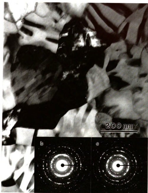
Figure 3-17. TEM BF image and the associated SADP's taken from the midplane of the film H773. The SADP (b) and (c) were recorded at a tilt of 0 and 30 degrees, respectively. The micrographs show coarse precipitates and the random grain orientations.
