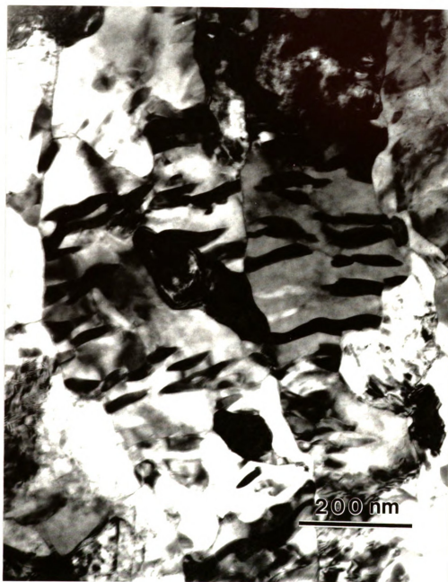
Figure 3-54. TEM bright-field images from deformed film H723. Just like its undeformed structure, well-defined precipitate particles and grains without any dislocation can be seen.
