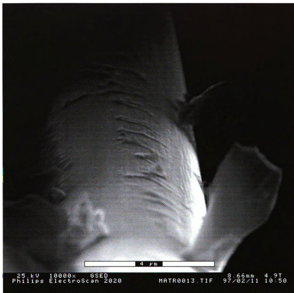
Figure 7-7 Matrimid® 5218 Sizing on an IM7 Fiber Surface
