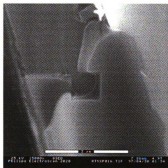
Beam Damaged RTV Sizing Showing Rubber-Like Properties
