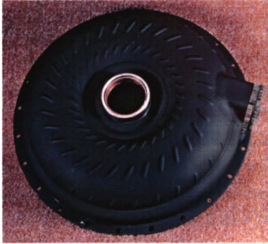
Figure 10. View of impeller half of converter with side window installed
