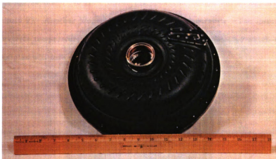
Figure 8. View of impeller half of converter with front window installed
