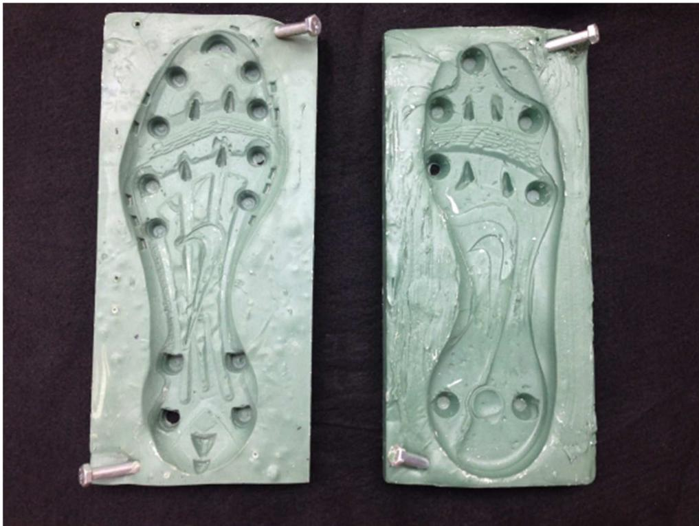
**Figure 4-3** Football cleat mold made of epoxy resin used to fix the shoe to the testing fixture
