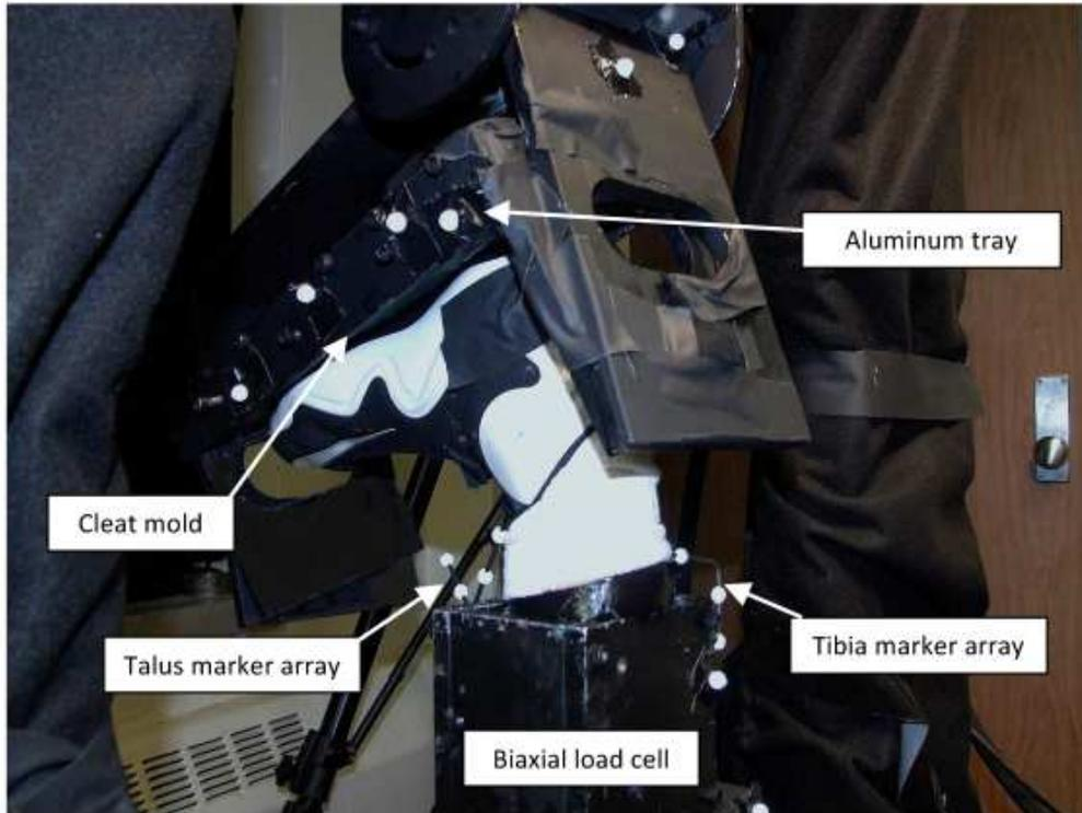
**Figure 4-4** *The experiments were performed on a biaxial testing machine with the motions of the talus and tibia tracked by a 5-camera motion capture system.*
