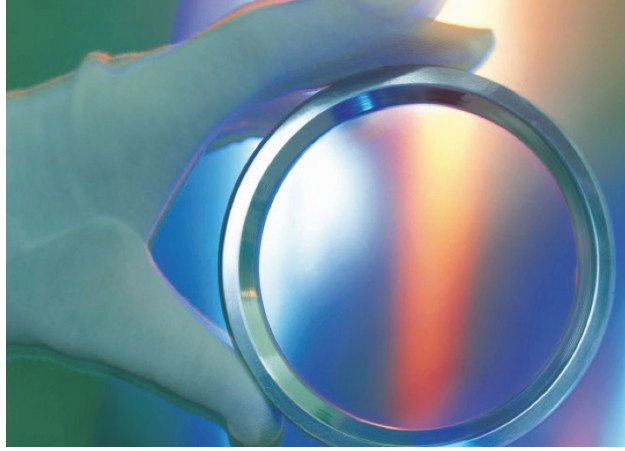
Figure 1.1 Mounted optical grade polycrystalline diamond window, ready for use in high power CO_2 laser optics [7]
