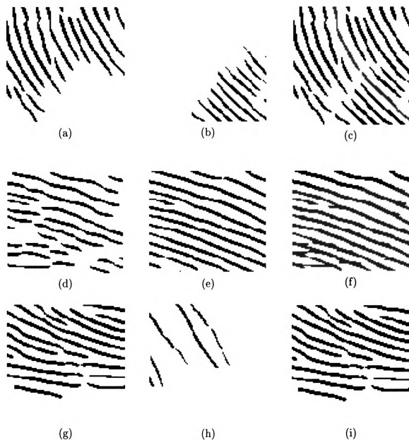
Figure 5.9: Intuitive meaning of the voting algorithm; here for simplicity, we assume that the input image is decomposed into two filtered images; (a)-(c) correspond to rule 1; (d)-(f) correspond to rule 2; (g)-(h) correspond to rule 3; the left two columns show the inputs to the voting algorithm while the third column shows the voting results.
