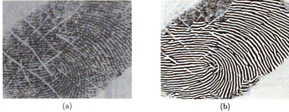
Figure 1.5: Fingerprint image enhancement: (a) corrupted image; (b) enhanced image.
