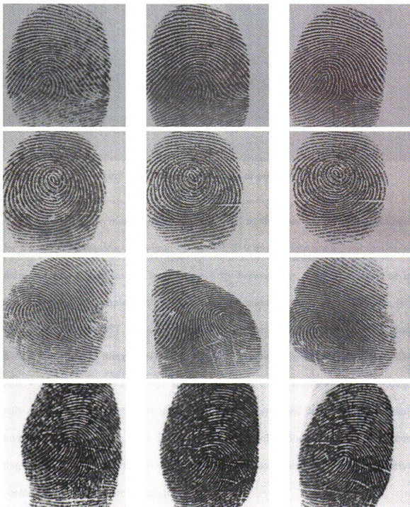
Figure 9.1: Fingerprint images captured with a scanner manufactured by Digital Biometrics; the size of these images is 640 \times 480 ; images in each row are from the same finger.
