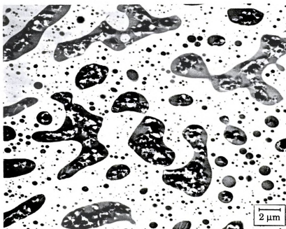
Figure 83: TEM picture of CA/SMA-R/DMAp 70/30/0.01 after extrusion (sectioning perpendicular to the flow direction).
