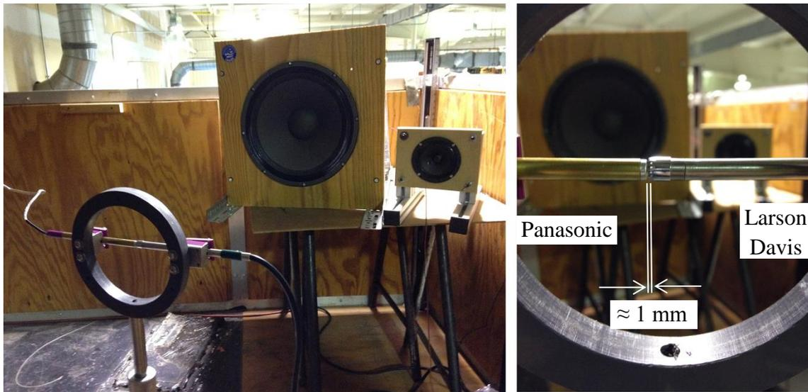
**Figure 2-13 Panasonic calibration setup**
