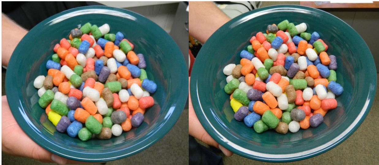
Figure 4.10. Side-by-side color comparison, where the current F32T8 lighting technology is shown in a, and the perspective LED lighting technology is shown in b
