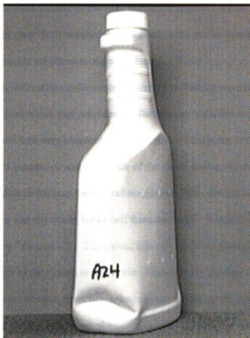
Figure 11. Bottom dent in anti-bacterial cleaner bottle placed in storage at 120 °F.
