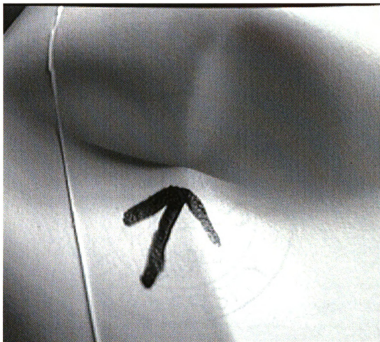
Figure 23. Detailed view of anti-bacterial cleaner bottle shoulder dent of Figure 8.
