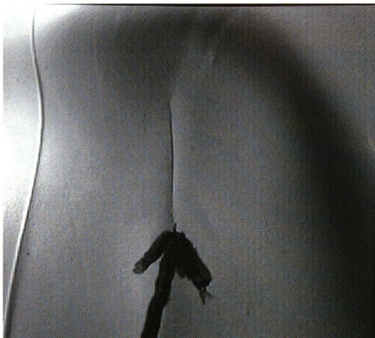
Figure 22. Detailed view of anti-bacterial cleaner bottle shoulder dent of Figure 7.
